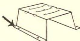
The lower flanges are provided with nail holes. The forms are accurately and firmly held in place on the centering.
