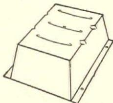
Meyer Tapered Endforms increase the width of the joist and provide a compression flange or tee for the supporting beam or girder, and DO NOT increase the area of concrete below the neutral axis.
