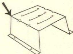
The square corners on Meyer Steel Forms save concrete and insure a clean cut job without jeopardizing the strength of the beams.
