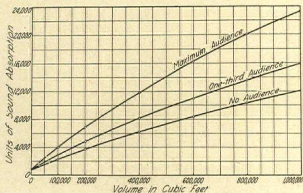
FIG. 6. AMOUNT OF SOUND ABSORBENT NEEDED FOR DIFFERENT SIZED ROOMS
