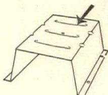
The ingeniously designed stiffening ribs in the top surface of Meyer Steel Forms secure the necessary rigidity to withstand heavy trucking loads. They also prevent sagging of the form under weight of concrete and insure a neat job.
