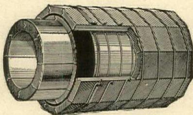
Wyckoff's Underground Improved Steam Pipe Covering is built up of Cypress, the Wood Eternal, or White Pine. The Inner Shell is made of Two-inch staves drawn together by heavy tension in tubular shape and firmly bound with extra heavy steel wire, bound spirally with extra wrapping at each end, insuring strength and compactness.
