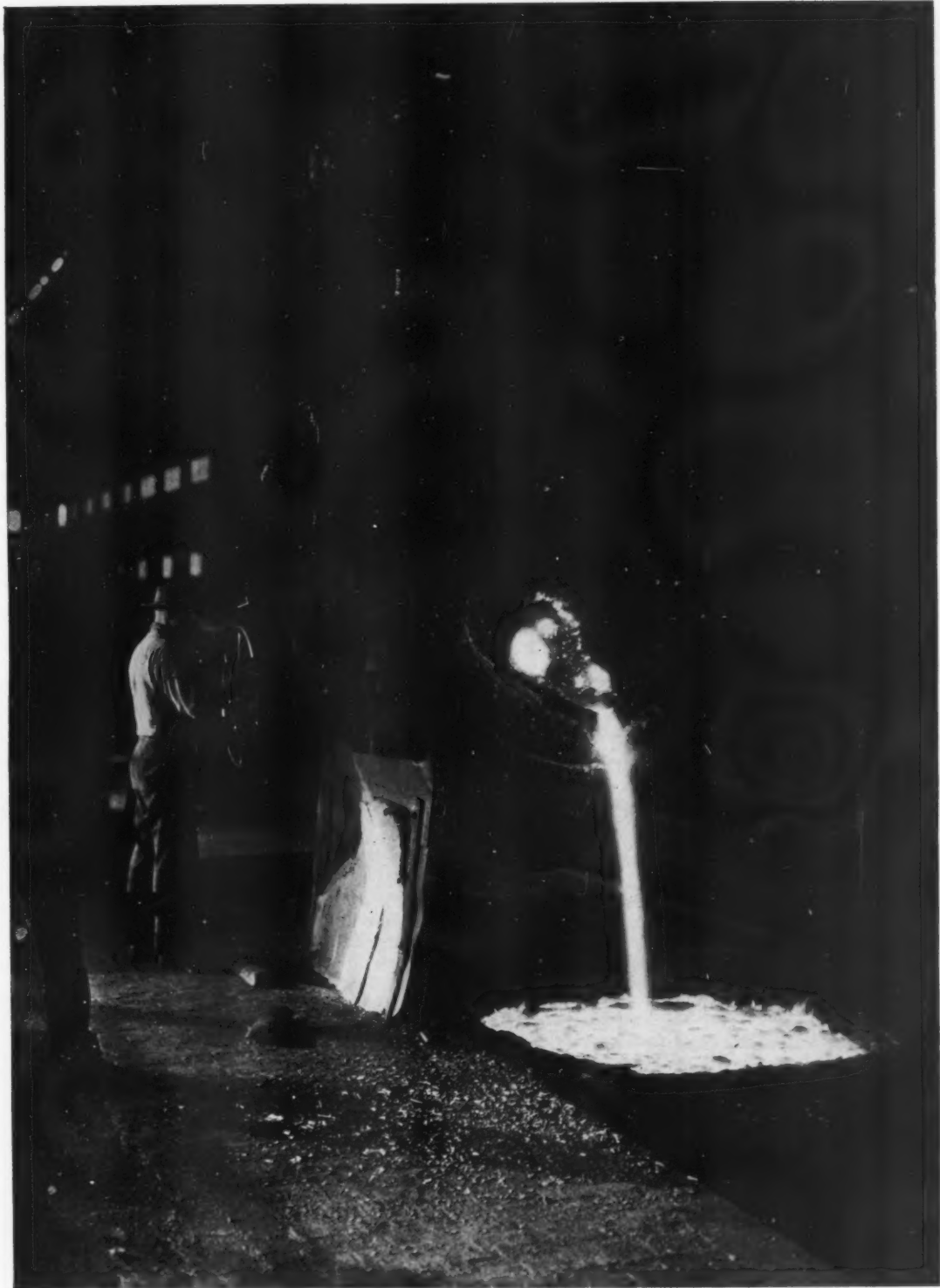
"PUDDLING" IS THE BASIS OF THE NEW ASTON PROCESS OF MAKING WROUGHT IRON. THE MOLTEN METAL IS POURED INTO A BATH OF SILICATE SLAG. THE RESULTING "PUDDLE BALL" CONSISTS OF NUMEROUS PEA-SIZED GLOBULES OF PURE IRON, COATED WITH SILICATE SLAG.
