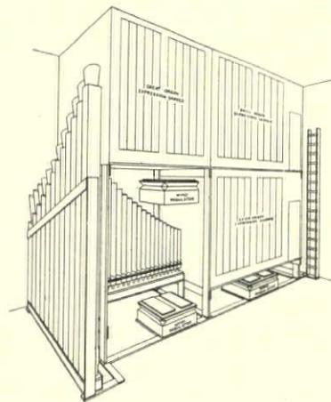
FIG. 8 — THREE MANUAL AND PEDAL ORGAN. THIS IS USUALLY A BETTER ARRANGEMENT AS TO SPACE THAN THAT SHOWN IN FIG. 7
