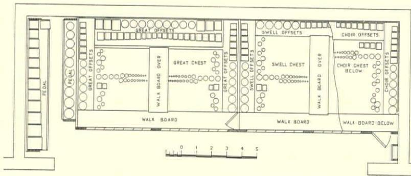
FIG. 9—PLAN OF THREE MANUAL AND PEDAL ORGAN SHOWN IN FIG. 8.
