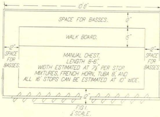
FIG. 1—PLAN OF TYPICAL ORGAN ENCLOSED IN SWELL BOX
