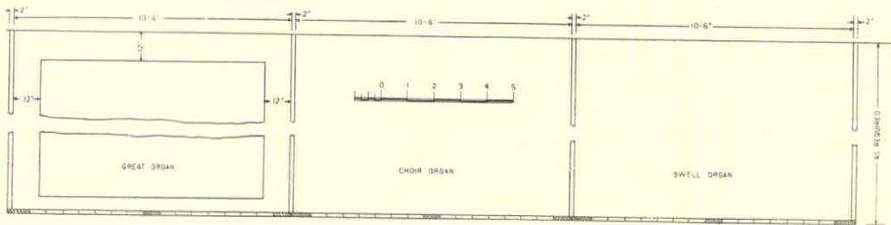
FIG. 7—THREE MANUAL ORGAN IN ONE CHAMBER. TRIAL ARRANGEMENT. PEDALS ARE NOT SHOWN
