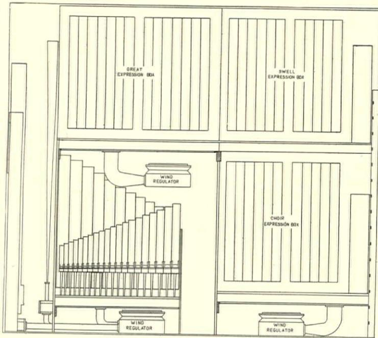
FIG. 10—ELEVATION OF THREE MANUAL AND PEDAL ORGAN SHOWN IN FIG. 8
