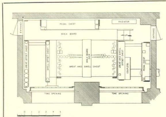
FIG. 3—PLAN SHOWING SMALL ORGAN ENCLOSED IN ORGAN CHAMBER. ENTIRE ORGAN CONSIDERED AS ONE TONAL UNIT
