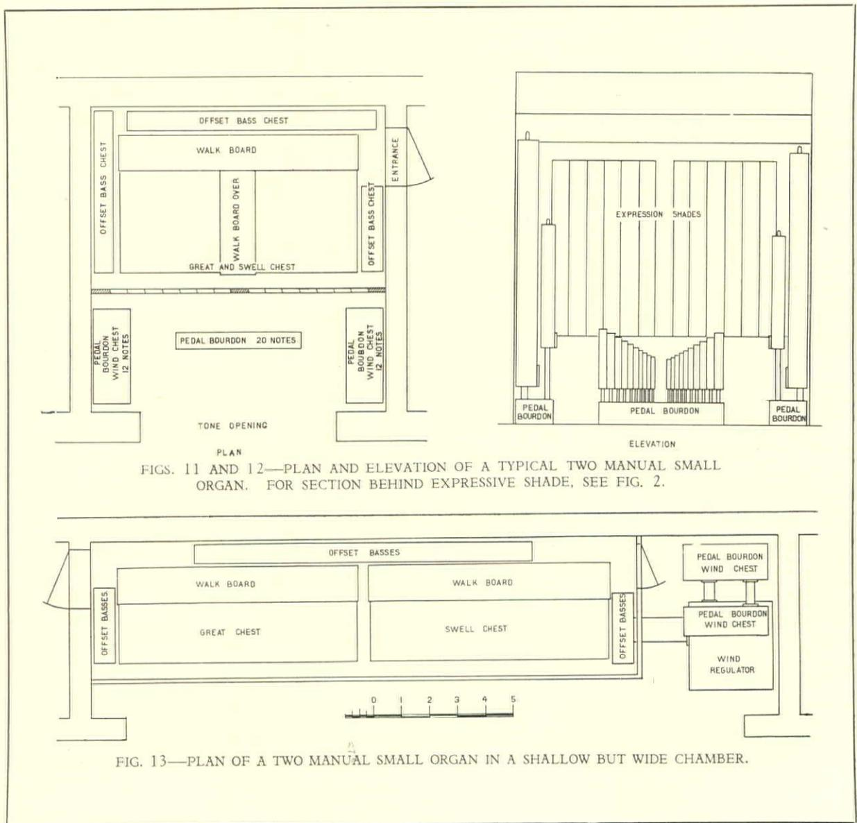
FIGS. 11 AND 12—PLAN AND ELEVATION OF A TYPICAL TWO MANUAL SMALL ORGAN. FOR SECTION BEHIND EXPRESSIVE SHADE, SEE FIG. 2.
