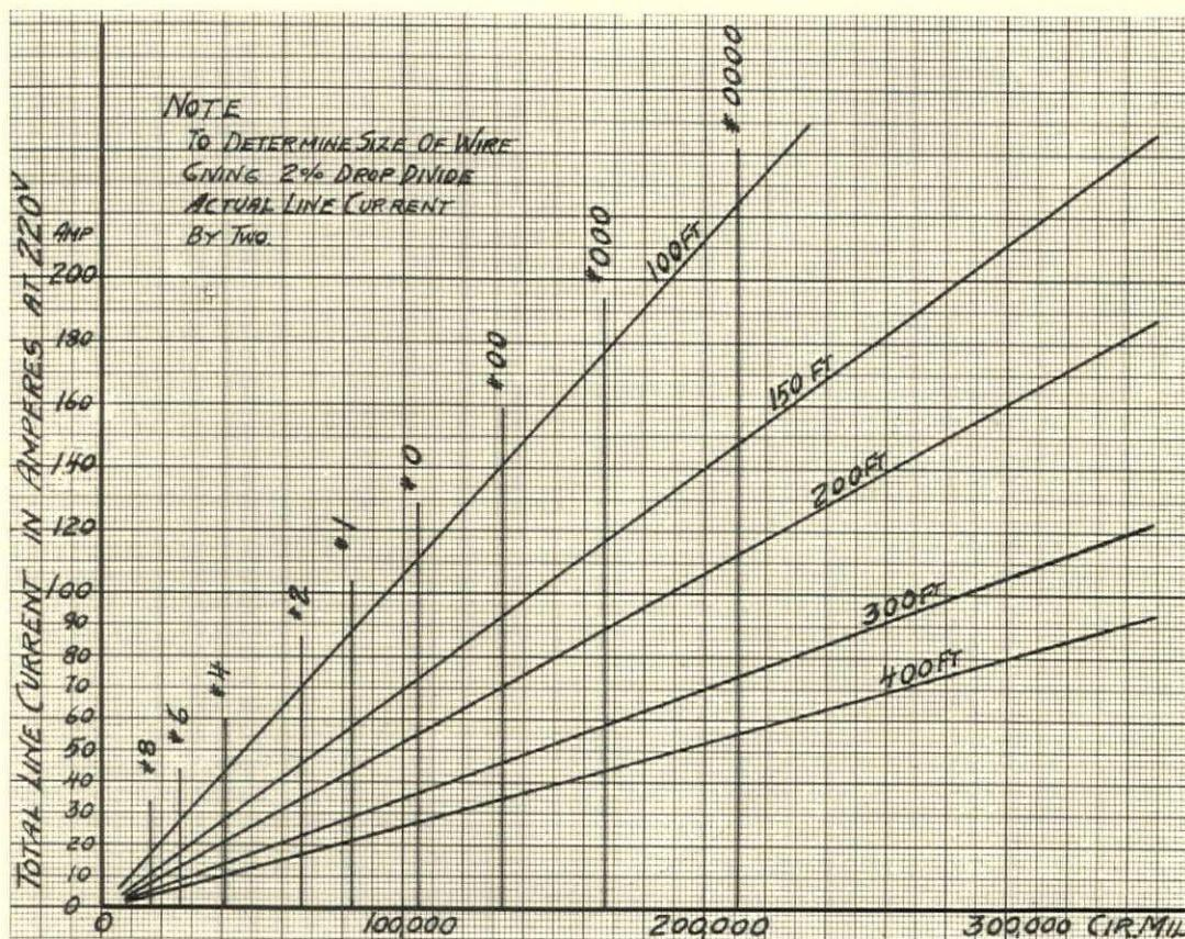
WIRING CHART SHOWING SIZE OF WIRE FOR VARIOUS CURRENTS AND DISTANCES ASSUMING ALLOWABLE DROP OF ONE PER CENT BETWEEN INCOMING SERVICE AND X-RAY MACHINE
