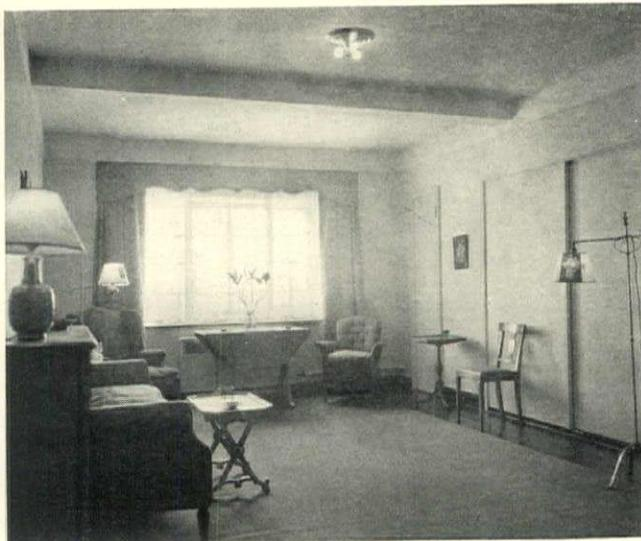
*A one room apartment. The doors of the doorbed, shown at the right of the room, slide on a track notched to take the down-sprung bed supports, thus permitting the doors to be closed when the bed is in use*
