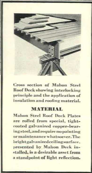
Cross section of Mahon Steel Roof Deck showing interlocking principle and the application of insulation and roofing material.
