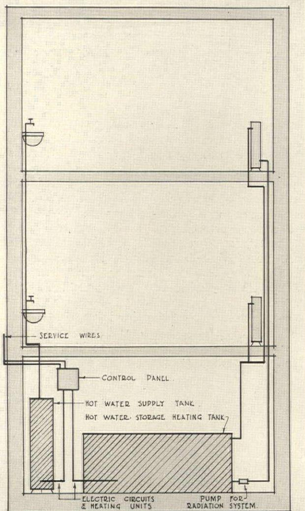
Diagram showing the essential features and typical arrangement of units of an "off peak" electrical heating system
