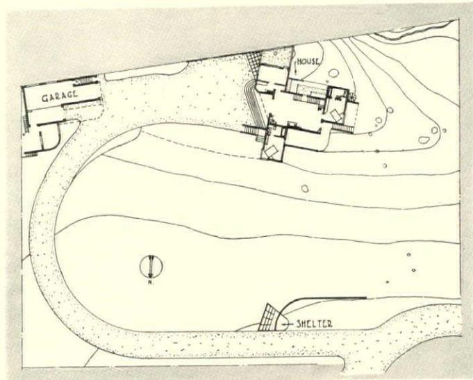
Topographical map of the two-acre plot on which the Porter house is located. The house is planned to conform to existing grades to avoid terracing
