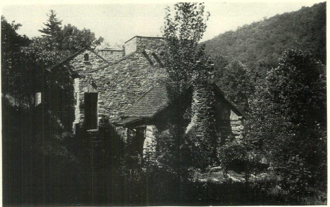
Unskilled labor built this house with native and old materials. Walls, salvaged brick and stone picked up on the site. Heavy timber framing, hand-hewn shingles, hand-forged hardware. Above: house from the drive; below, old log cabin, now used as study. Facing page, above: sun terrace; below, right, entrance detail
