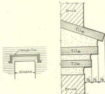
Elevation and detail section of label mould
