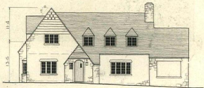
Exterior walls, local limestone ranging in color from cold to warm buff gray. Vertical stone joints filled flush with mortar and surface brushed with a gunny sack. Interior walls, dull ivory, palm-finished plaster. Ceilings, exposed timbers, rough sawn ceiling boards. Floors, oak, random widths. Fireplace facing, common Holland brick. Trim, wormy chestnut. Window sills, kiln run floor tile. 34,500 cubic feet. Cost 53.5 cents per cu. ft. Built 1930
