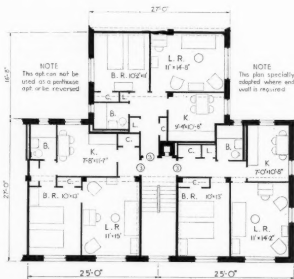
3 UNIT 3-3-3-A Total gross area per unit - 1818 sq. ft. Average gross area per room - 202 sq. ft.
