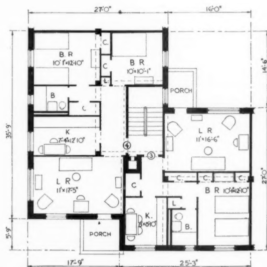
29 CORNER UNIT 3-4 Total gross area per unit - 1440 sq. ft. Average gross area per room - 205 sq. ft.
