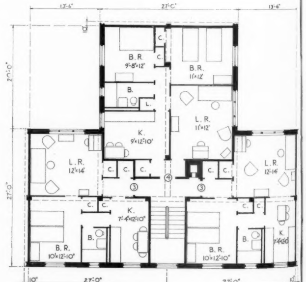
4 UNIT 3-4-3 Total gross area per unit - 1998 sq. ft. Average gross area per room - 200 sq. ft.
