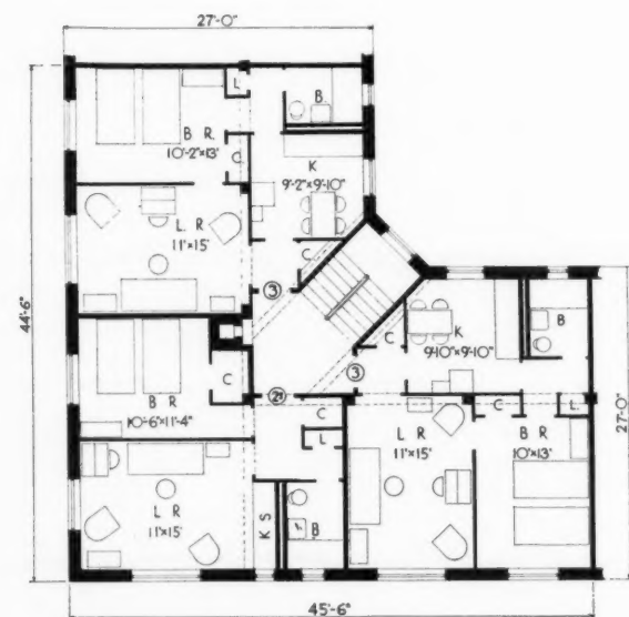
28 CORNER UNIT 3 2s 3 Total gross area per unit - 1711 sq. ft. Average gross area per room - 214 sq. ft.
