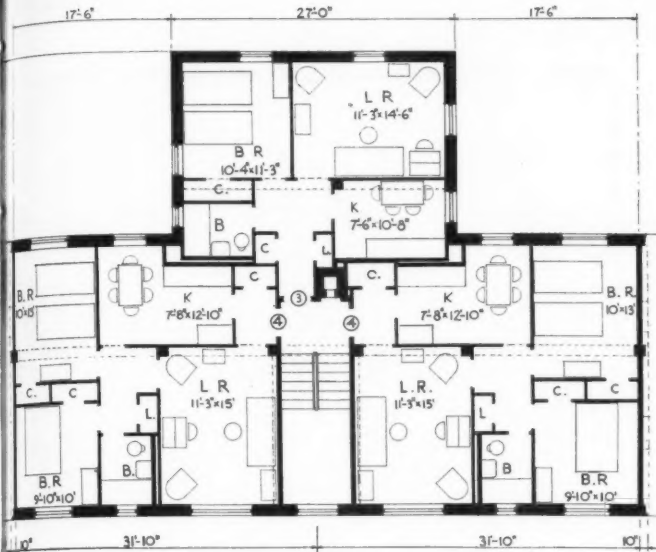
11 UNIT 4 3 4 Total gross area per unit - 2146 sq. ft. Average gross area per room - 195 sq. ft.
