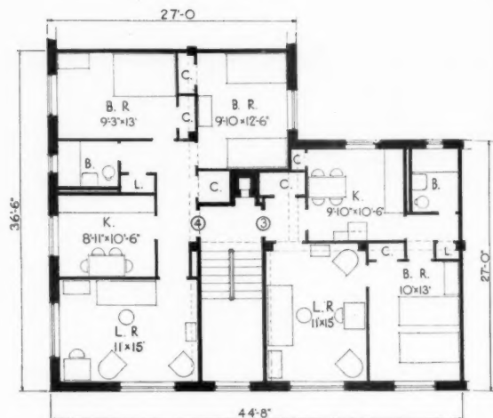
25 UNIT 3-4 Total gross area per unit 1462 sq. ft. Average gross area per room 205 sq. ft.
