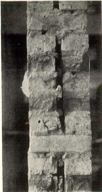
**Figure 4 . . .** Broken section of 8-inch brick wall as laid up by a mason following common practice with a harsh mortar. Unfilled joints form reservoirs in which water may collect, eventually penetrating to the interior
