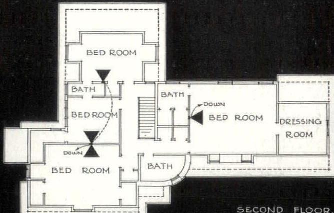
LEGEND    ◀ TELEPHONE OUTLET    - - - - - CONDUIT    [PB] PULL BOX    [PC] PROTECTOR CABINET
