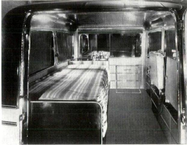
A "hospital room on wheels" recently placed in service in New York, was designed by Irvin L. Scott of Joseph Urban Associates. This latest word in ambulances has controlled heat and ventilation, hot and cold running water, one-way-vision windows, sound-proof walls and floors of rubber in addition to adjustable beds and three armchairs for attendants. The color scheme is terra cotta, light green and chromium
