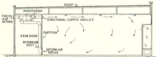
Taking but small space, a Moditherm can be easily installed. Sketch above shows unit located at ceiling line in rear room of average size store. Conditioned air is discharged directly into store space without use of ducts.
