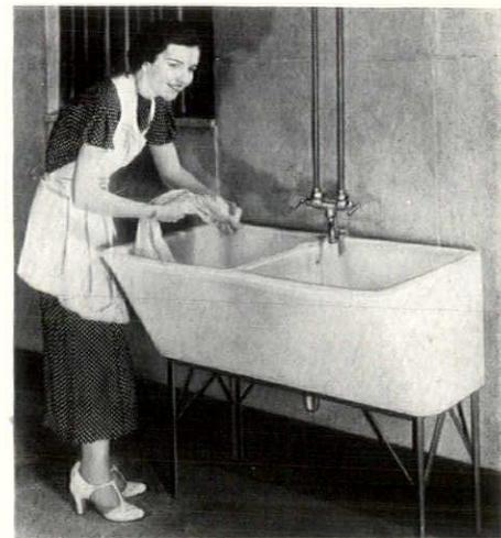
Crane Company, Chicago. It is of one-piece construction and is made of hard, durable porcelain. The corners are rounded for ease of cleaning and its glass-like surface is claimed to be unaffected by strong alkalis, dyes or acids (except hydro-fluoric). The double swinging spout faucet is installed above the rim of the tub to prevent back-siphonage. It may be had either in white or buff color and in both single and double compartments. **557M**
