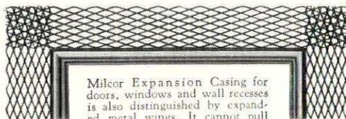
Milcor Expansion Casing for doors, windows and wall recesses is also distinguished by expanded metal wings. It cannot pull away during settlement and will not leave cleavage cracks.
