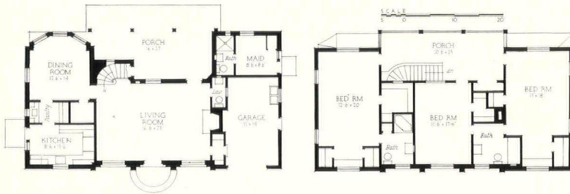
A modernized Colonial type house of reinforced concrete block with a stucco finish and run stucco molds. The roof is of black asbestos shingle and sash is of steel. The open porch has a brick floor and the glazed second story porch floor is of tile
