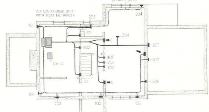
Figure 1. Layout for a Direct Fired System. The house plan is selected as representing a fairly typical problem—the work of William Paries, architect
