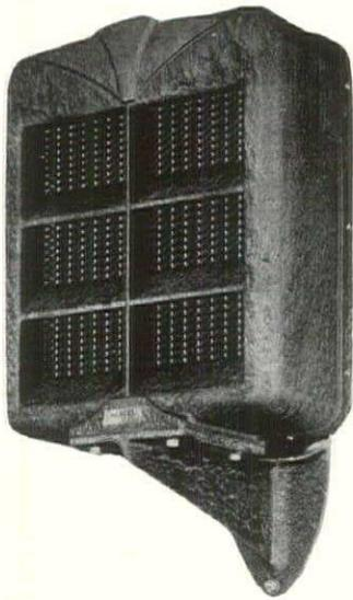
and the low heat for maintaining the temperature. This new unit is a complete electric heating plant in itself. No piping is necessary, and it can be installed any place by connecting it to the electric circuit. The heater has an all-copper core with cast top and bottom tanks. Electric immersion-type heating elements enclosed in
