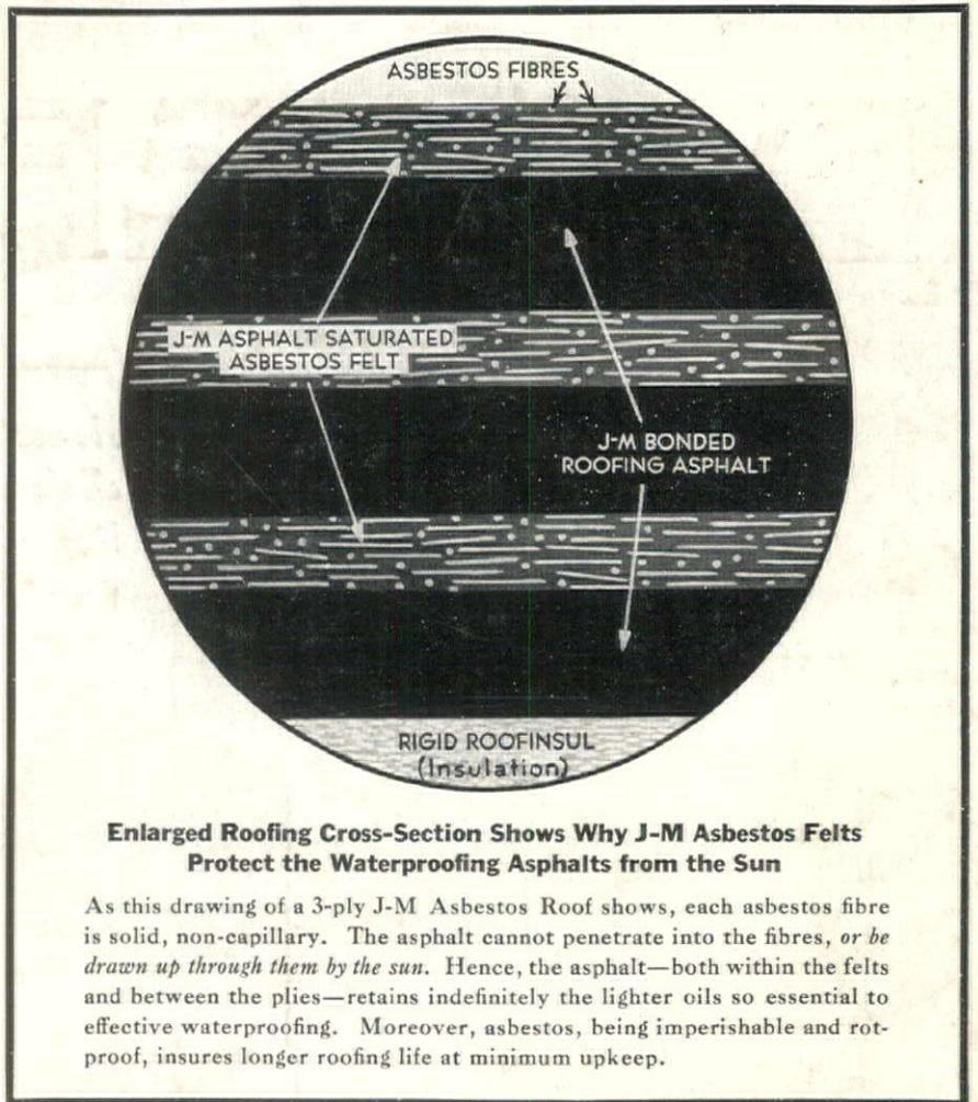
**Enlarged Roofing Cross-Section Shows Why J-M Asbestos Felts Protect the Waterproofing Asphalts from the Sun**
