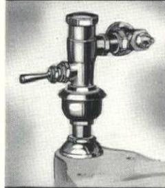
DELTA Flushing Valve with VIGILANT Vacuum Breaker. Quantity of water delivered adjustable. Valve closes even though handle is held down. Vacuum breaker prevents back siphonage. Applicable to any closet bowl and flushing valve.
