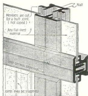
Typical Capped-Joint Construction.
