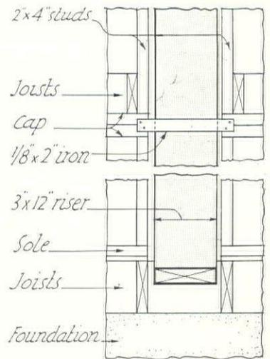
Some of the structural details in the best duct work practice: At the left, a variation of the sill, introducing a riser without serious cutting; above, damper details and a framing scheme in combination with a steel beam that turns up a riser without cutting; at right, the use of a reinforcing iron plate where a duct cuts through a partition cap
