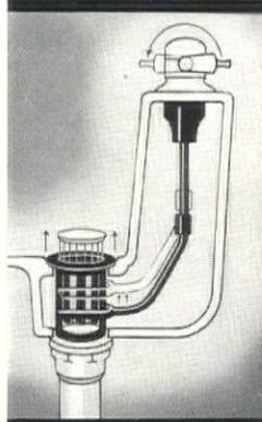
ACCESSO Bath Waste. When closed, held tight by the weight of water. Contamination of newly drawn water impossible.
