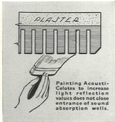
Painting Acousti-Celotex to increase light reflection values does not close entrance of sound absorption wells.
