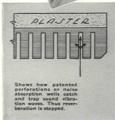
Shows how patented perforations or noise absorption wells catch and trap sound vibration waves. Thus reverberation is stopped.
