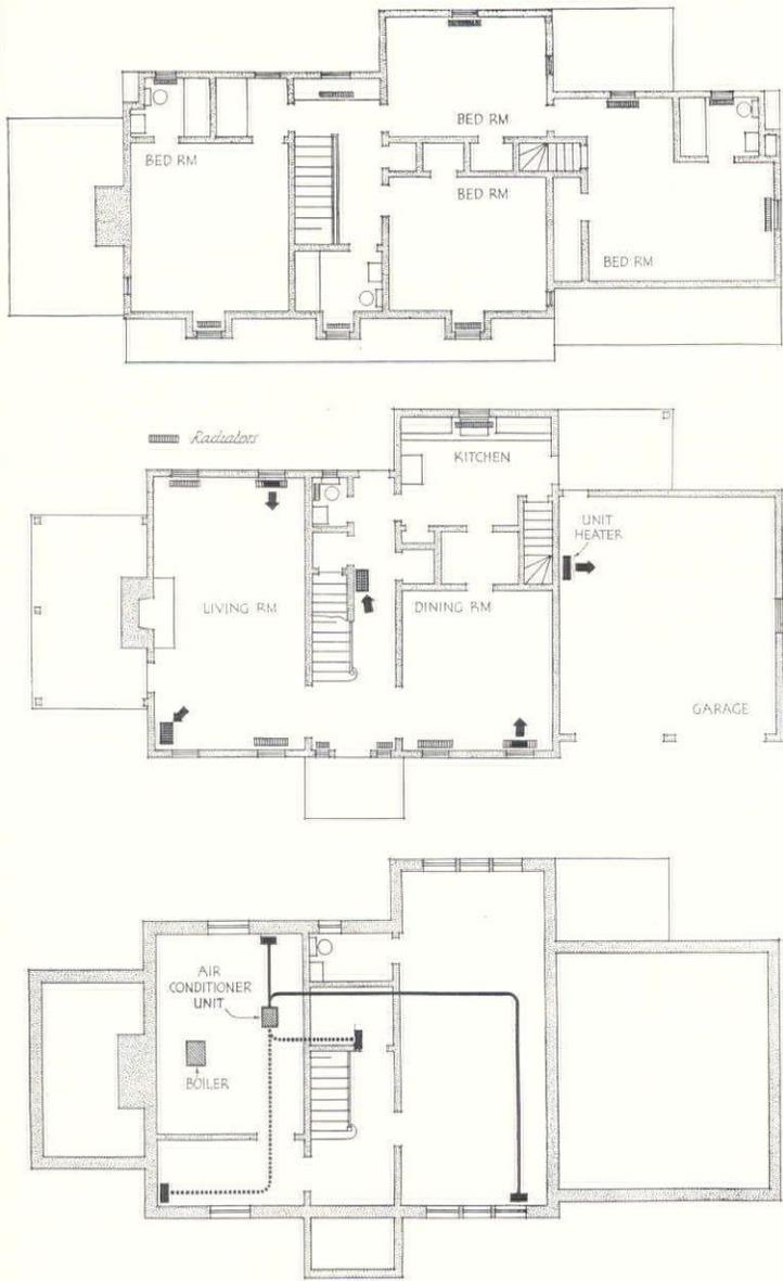
Figure 3. Layout for an Auxiliary System in the same plan as that used for the other two systems
