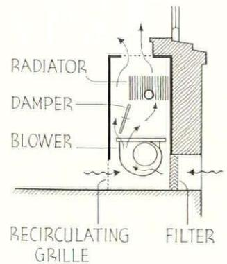
UNIT VENTILATOR WITH HEATER AND FORCED CIRCULATION
