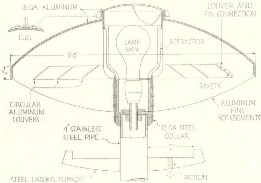
This hooded fixture was designed for the illumination of parking spaces in the vicinity of the dam, where spill of light beyond the area to be lighted is objectionable. The hood and louvers cut off direct view of the refractor beyond that area. Light distribution within those limits may be controlled by the choice of the refractor and by adjustment of the bulb center. The fixture may be relamped from the top
