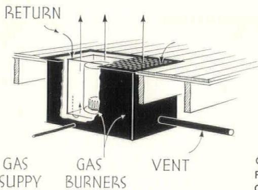
**GAS-FIRED FLOOR FURNACE OF RECIRCULATING TYPE**
