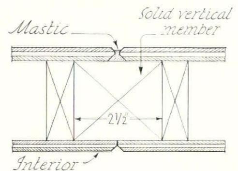
Figure 1 (left). Section showing typical assembly of floor, wall and roof panels. Figure 2 (above). Plan showing solid vertical member fitted into the grooves on the sides of adjacent wall panels
