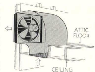
ATTIC FAN FOR COOLING WITH NIGHT AIR
