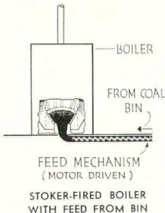
STOKER-FIRED BOILER WITH FEED FROM BIN
