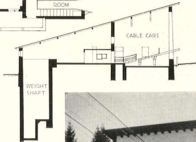
Essentially merely a waiting room and ticket office, the first station is characteristic of the architectural treatment of all three. Built of reinforced concrete with cement-finished walls of brick and stone, its forms recall local precedent. Wood trim is stained dark brown and the steep pitched roofs are of metal
