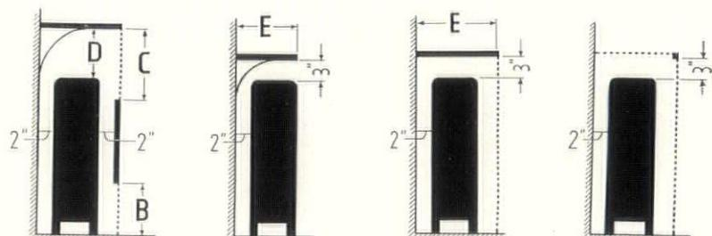
No change when B = 80% of A as in preceding figures; C = 150% of A and D = A
