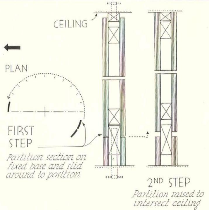
A semi-circular screen of wood separating the dining area from the living room constituted a minor engineering problem because the large radius required that prefabricated sections be ingeniously assembled on the job. Below, two other examples of the use of glass, (2) mirrored partitions, and (3) a metal-framed clear glass windscreen.
