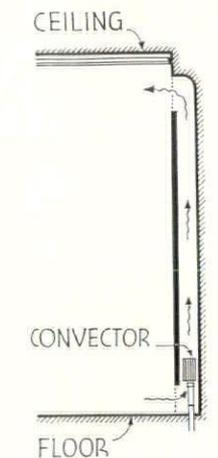
CONVECTOR WITH FLUE EXTENDED TO UPPER WALL
