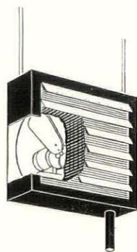
UNIT HEATER OR COOLER, SUSPENDED TYPE
