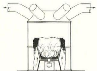
WARM AIR FURNACE WITH VERTICAL OIL BURNER
