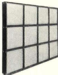
There are two types of DUST-STOP Filter Frames. The L-type consists of an assembly of interchangeable L-shaped members that may be assembled vertically or horizontally to provide capacity for any c.f.m. requirement.
