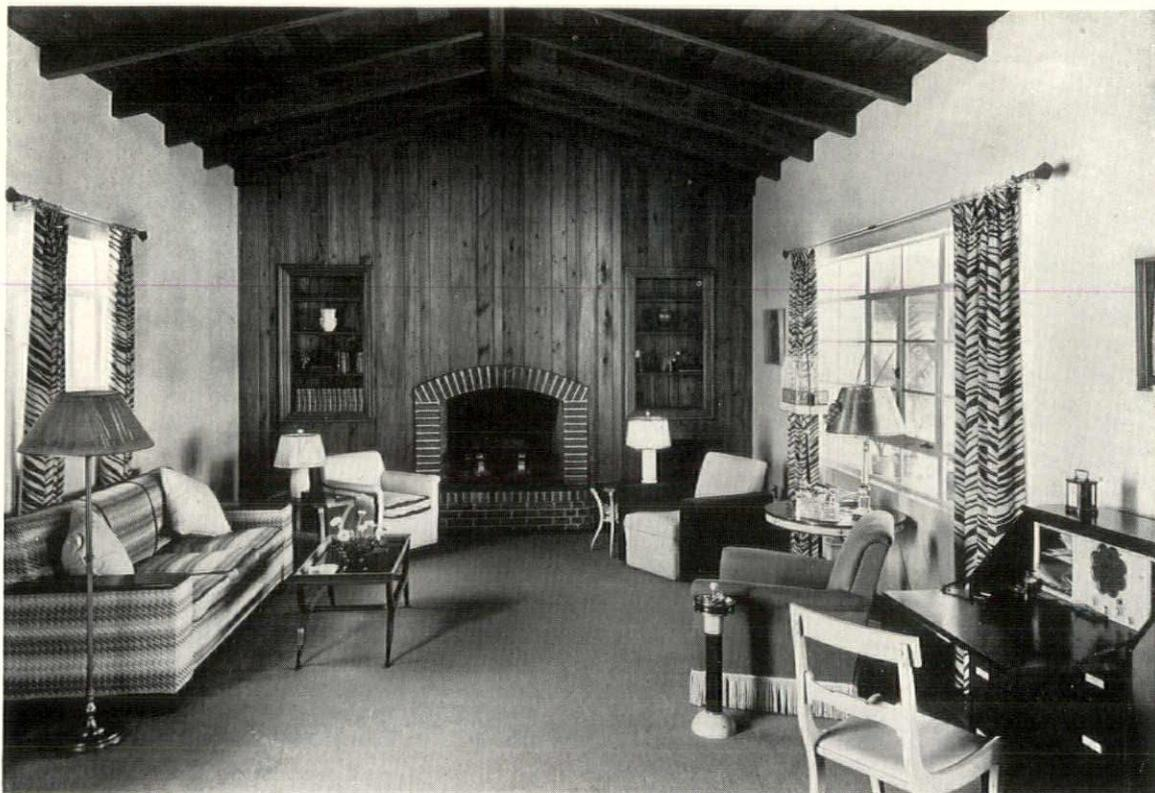
All interior trim, including ceiling and fireplace wall paneling, is of cypress. Flooring is of oak. The second floor exterior wall on the garden side (below) is of frame, sheathed roofing felt, metal lath and stucco. Porch flooring is of handmade Cuban tile on concrete slab.
