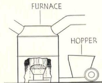
STOKER-FIRED FURNACE WITH HOPPER FEED
