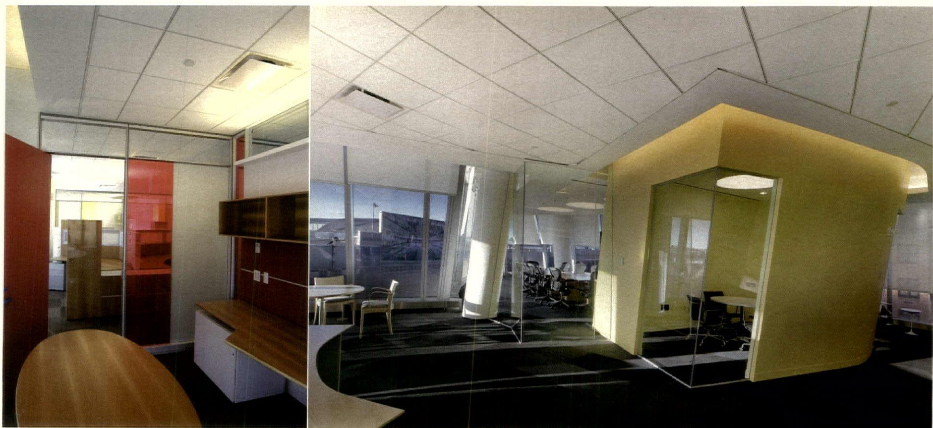
Private offices (left) have a modular aluminum-and-glass wall system that can conform to the IAC's irregular angles, which are the very elements Studios Architecture chose to play up in common spaces and conference rooms (right).
