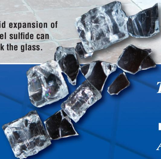
JEB offers 100% heat soak testing for 1/4" through 3/4" uncoated or pyrolytic low-e glass that is typically used in demanding or higher risk glazing applications.
