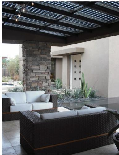
The National Association of Home Builders' 2009 New American Home show house in Las Vegas, designed by California-based Danielian Associates, integrates a new type of PV technology into its poolside trellis and awning structures. The bifacial panels manufactured by Sanyo produce power from both sides, resulting in a previously unattainable 23 percent energy-conversion efficiency.
