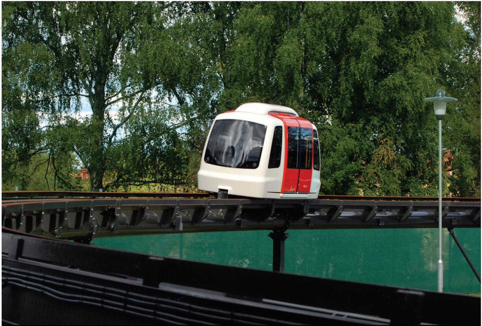
**Facing page:** The ULtra system planned for London’s Heathrow Airport will run rubber-wheeled vehicles along a concrete guideway.
