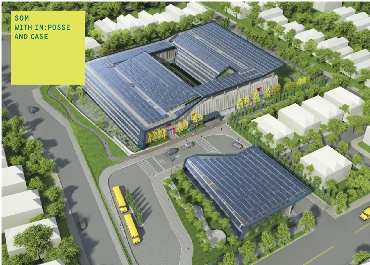
Above: Roof-mounted PV panels will produce all of the school's energy over the course of the year; facing page: Daylight floods interior corridors; bottom: East elevation.
