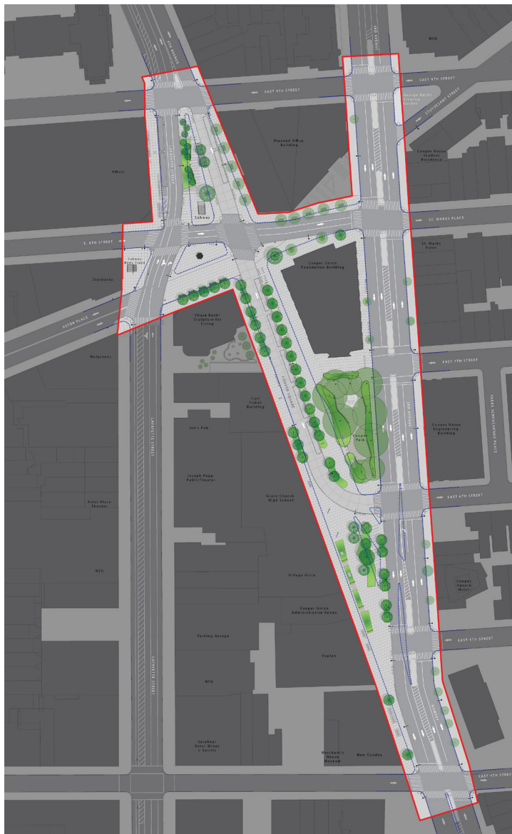
Opening page: A redesigned courtyard at Pace University, designed by AECOM, was rebuilt to capture stormwater through permeable pavement and an advanced cellular support system; Above and below: Astor Place and Cooper Square are being redesigned with massive bioswales and large tree pits.
