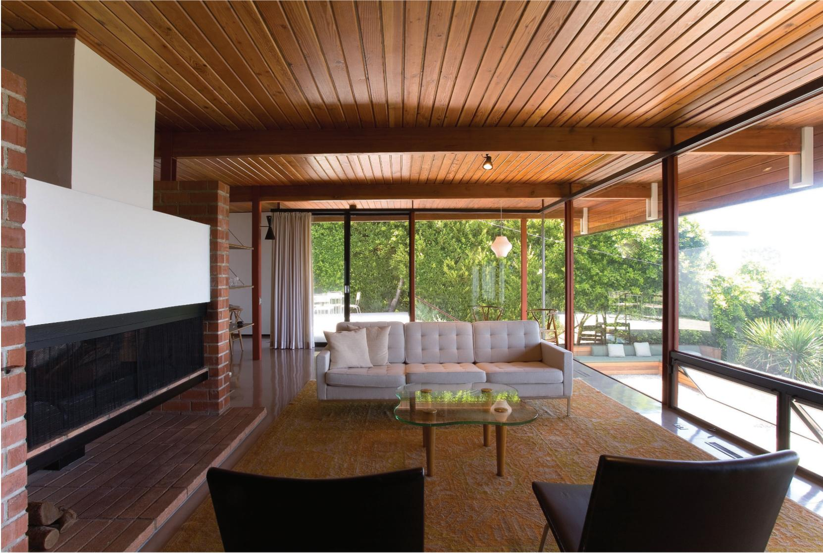
Craig Elwood's 1953 Johnson House (left) in Brentwood was restored by Du Architects, who stripped, polished, and replaced wood finishes and floors as necessary to maintain the original integrity of the house. Venice-based SH\_Arc replaced the wood, stone, plaster, and glass of Richard Neutra's 1956 Troxell House (below).
