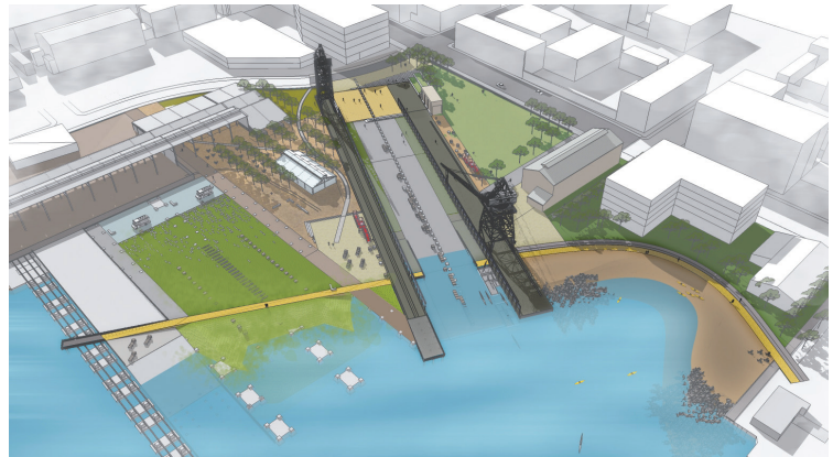
Below and opposite page, bottom: AECOM's Crane Cove Park in San Francisco is designed to flood, absorbing the brunt of a storm surge and protecting the populated area beyond
