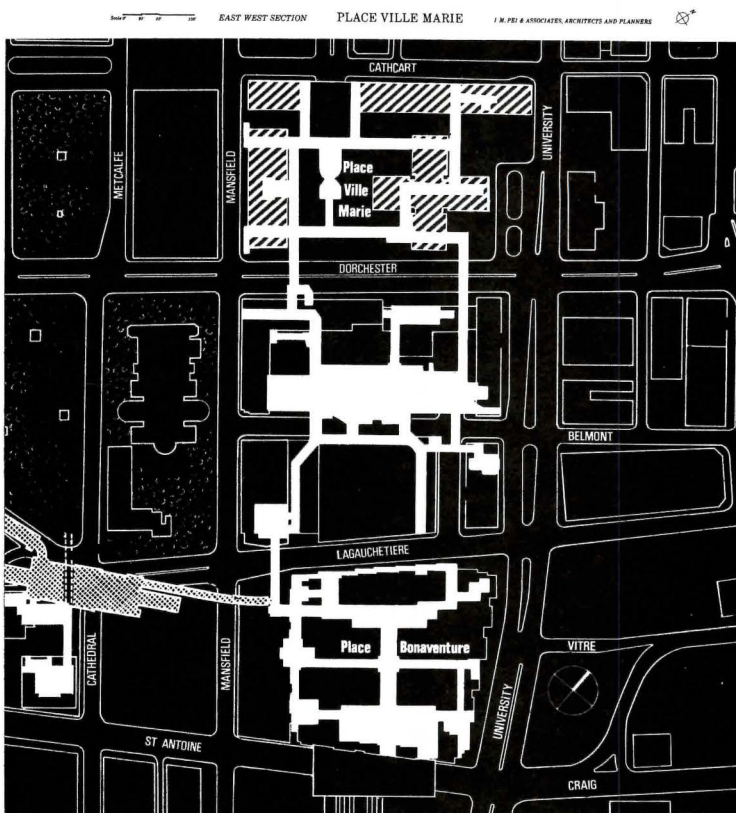
Above, Place Ville Marie, in Montreal, Canada, completed in 1962. The section on top shows the multi-level concourse below the main office tower; the plan shows the elaborate pedestrian concourses, highway tunnels, and metro lines that form PVM's infrastructure. Below, a view of the laboratories for the National Center for Atmospheric Research, in Boulder, Colorado, completed in 1966. Photograph: Ezra Stoller © ESTO
