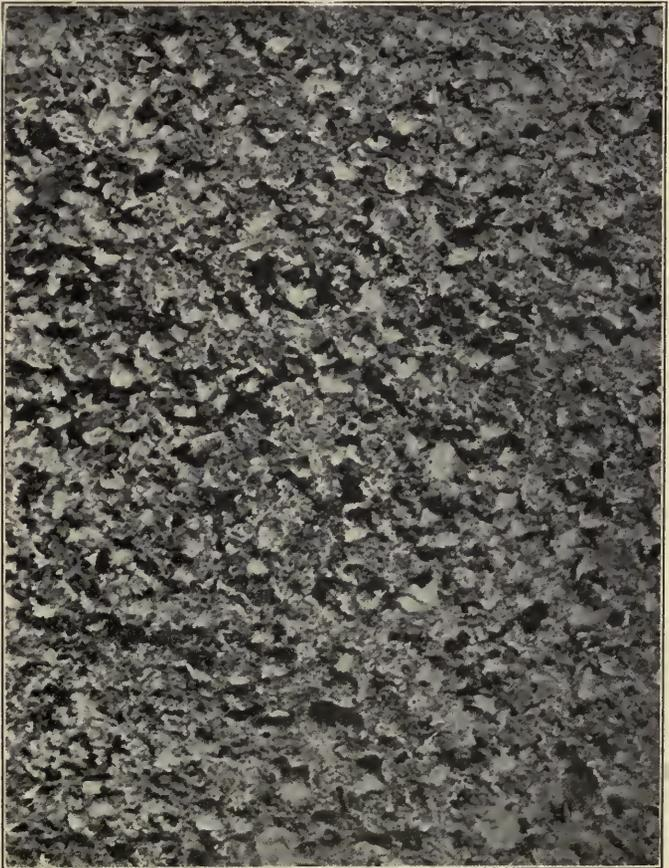
FIG. 10. SURFACE FINISHED BY PNEUMATIC HAMMER.
