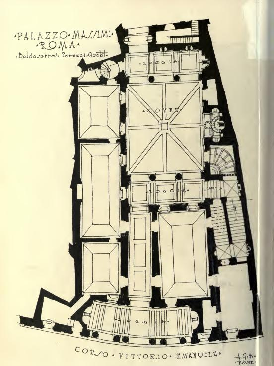
FLOOR PLAN—PALAZZO MASSIMO, BALDASSARE PERUZZI, ARCHITECT.
