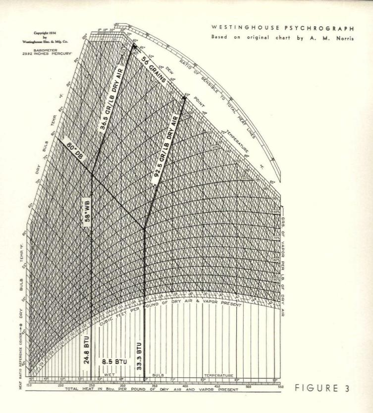
Given: Air at 80° dry bulb temperature and 58° wet bulb temperature.
