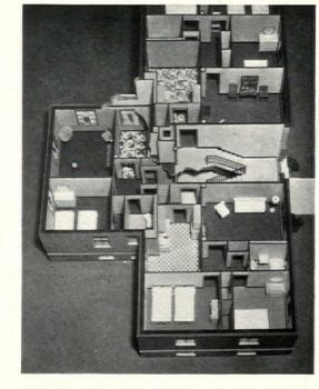
ONE OF THE TESTS APPLIED BY THE FEDERAL HOUSING DIVISION TO ITS ARCHITECTURAL PLANS FOR A PROJECT. THIS MODEL WAS BUILT TO ONE-HALF INCH SCALE FOLLOWING THE UNIT PLANS DISCUSSED IN THIS ISSUE OF THE ARCHITECTURAL RECORD.
