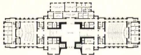
SECOND FLOOR PLAN: "The nine elevators and twelve of the twenty-four stair locations indicated on this level. Notice poché in Governor's Wing."
