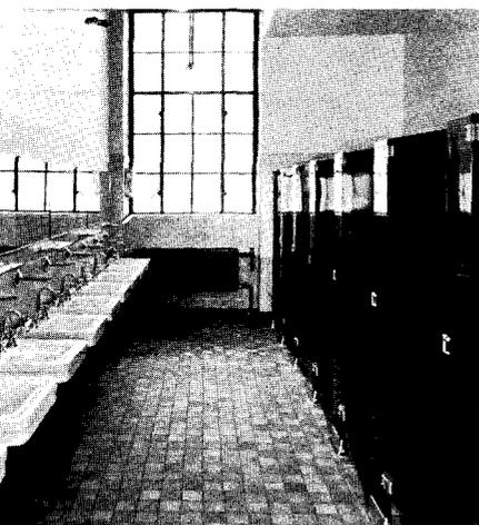
Washrooms. These vary from 120 sq. ft. to 150 sq. ft. in size. Lighting is standard direct. Walls, floor, base, and dado are of ceramic tile in shades of tan with white grout.
