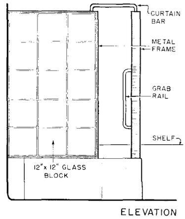
Glass-block partitions are used in the bathroom. Above is the corner tub, with side walls of glass block set in a metal frame, and a curtain bar provided over the opening.
