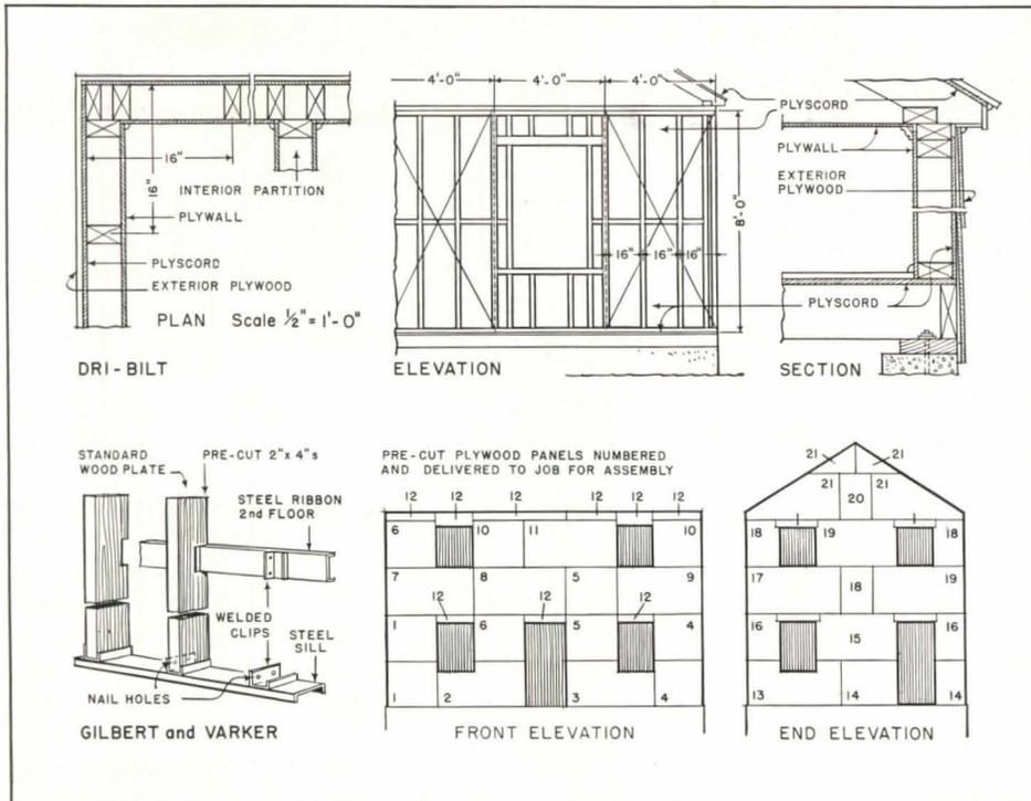
Dri-bilt system shown at top of sketch is sponsored by plywood manufacturers, and is essentially typical frame construction in which sheathing, subflooring, interior and exterior finish may all be of plywood. Methods developed by Gilbert and Varker (lower sketch) make
