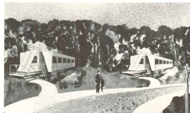
Architect Alfred Clauss of Knoxville, Tenn., offers the above scheme as one possible solution to defense housing needs. Necessary reductions in reproducing his drawings have obscured some details, but we hope not the essential idea. Size of shipping unit, according to Mr. Clauss, is 8 by 9 by 28 ft.; size of extended house, 22 by 11 by 28 ft.; estimated cost, \$900; weight, 6800 lbs.; erection time, one hour, with unskilled labor.
