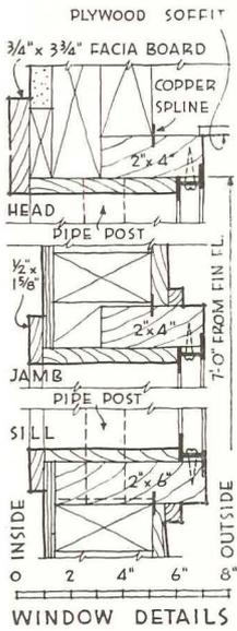
Windows are hung on a projecting wood frame—a simple and economical construction, according to the designer.
