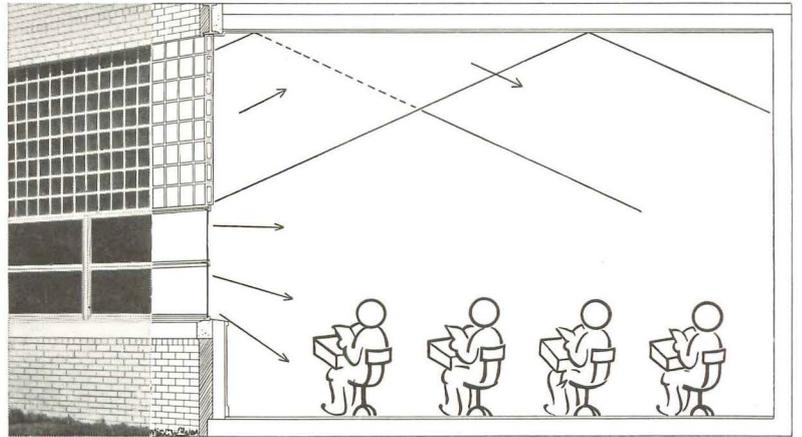
**BETTER LIGHT** for every pupil in rooms like this, with light-directional Insulux Glass Block above steel sash. The block throw light to ceiling, which reflects it evenly over room. Light-directional block are used on any exposure without objectionable glare.
