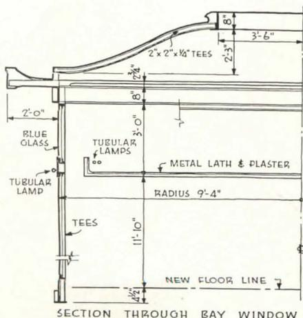
ORCHESTRA BAY in Zodiac room is suspended from an 18-ft. diameter steel ring cantilevered from the roof trusses, and projected 7 ft. beyond the building line. From the ring hang 3-in. steel tees which support the floor of the bay. Bay in Starlight room is similar, though rectangular and consequently simpler to fabricate
