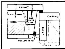
**PATENTED ROLLER-SEAL.** The York double seal provides two tough, pliable gaskets with sponge rubber cores and moisture-proof, grease-proof, wear-resisting coverings.
