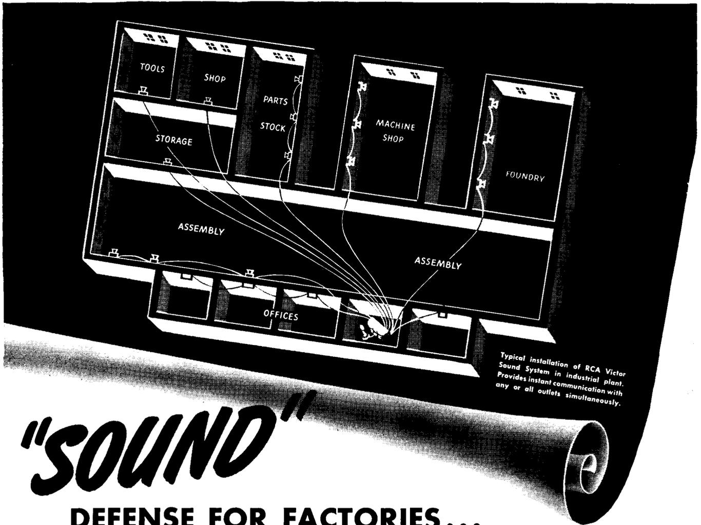
Typical installation of RCA Victor Sound System in industrial plant. Provides instant communication with any or all outlets simultaneously.
