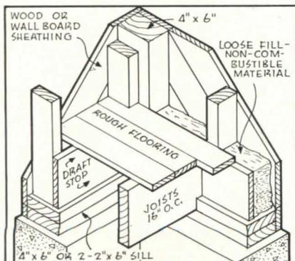
BRACED FRAME CONSTRUCTION
