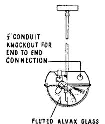
Both direct and indirect lighting is provided when CL-110 units are suspended from the ceiling.
