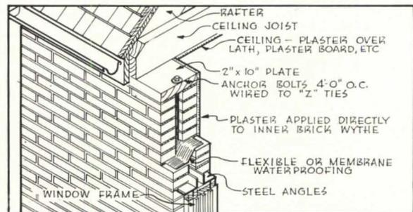
BRICK CAVITY WALL - SECTION THROUGH
