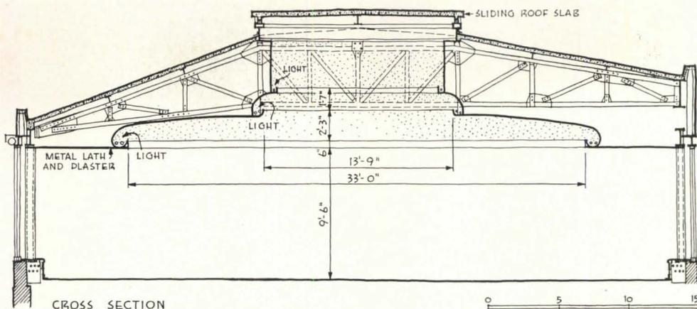
SECTION at right shows sliding roof directly over the circular Zodiac bar, and illustrates design of the trusses used to span from wall to wall. In addition, it demonstrates the way in which changes in ceiling level, etc., delimit various areas without using actual partitions
