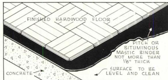
WOOD FLOOR OVER CONCRETE IN MASTIC
