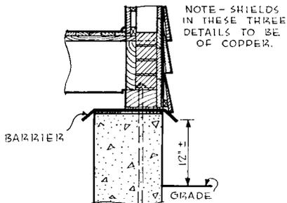
BARRIER SHIELD APPLIED TO FRAME CONSTRUCTION
