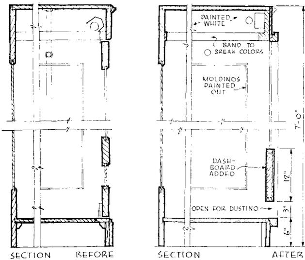
TYPICAL REMODELED CASE (above). Almost as much material was removed as was added. Receding wood and glass doors with their mechanisms and tracks were removed. A new cornice was added with a groove provided for cut-out letters. A dash board just above the base gives an even hem for dresses on display, conceals lighting and facilitates dusting
