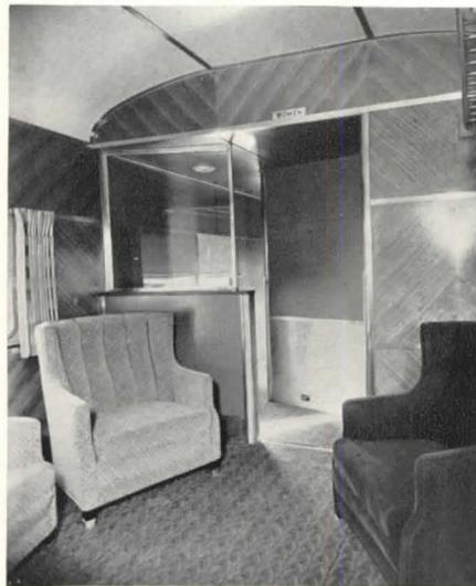
rents from the aerofuse outlets in the ceiling. Unbreakable glass is used at the door of the parlor car, which makes it possible to see down the passage from the car and into the car from the passageway. The glass panel is framed in stainless steel and the fin partition on which it rests has a stainless steel corner and a stainless steel base and a panel of bright color
