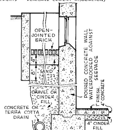
CONCRETE FOUNDATION WALL WITH AREA
