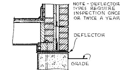
DEFLECTOR SHIELD APPLIED TO BRICK VENEER CONSTRUCTION
