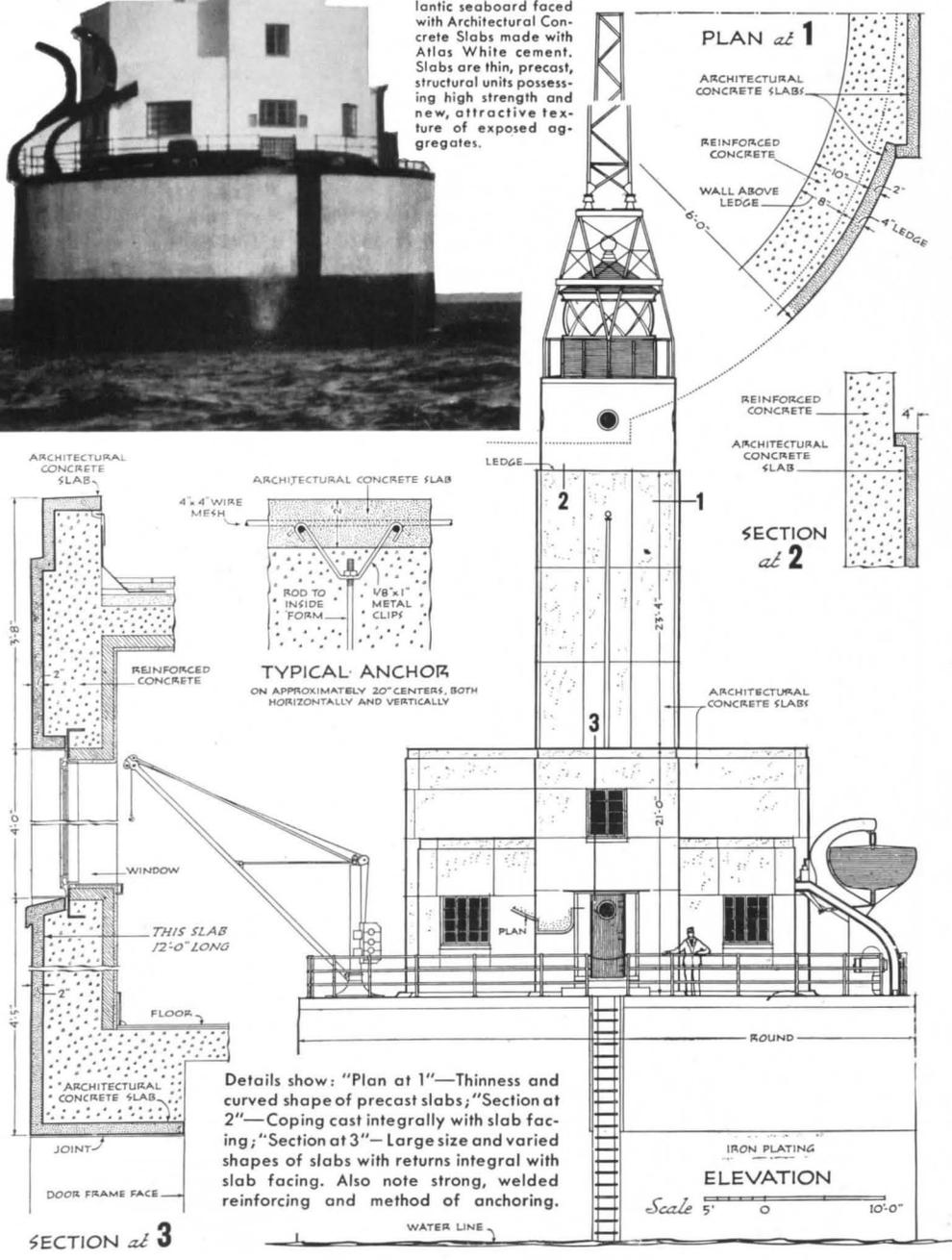
Details show: "Plan at 1"—Thinness and curved shape of precast slabs; "Section at 2"—Coping cast integrally with slab facing; "Section at 3"—Large size and varied shapes of slabs with returns integral with slab facing. Also note strong, welded reinforcing and method of anchoring.
