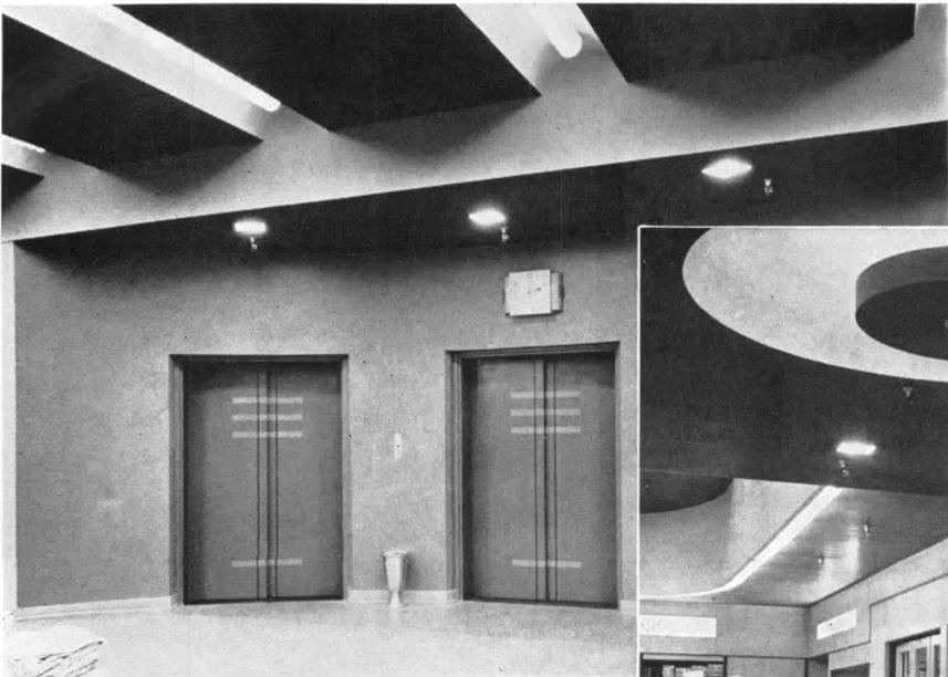
View (above) from first-floor elevator landing to main entrance on Orleans St. Floor here is terrazzo; store equipment fixtures are of bleached pin oak and prima vera. A complete sprinkler system was installed; pipes are concealed
