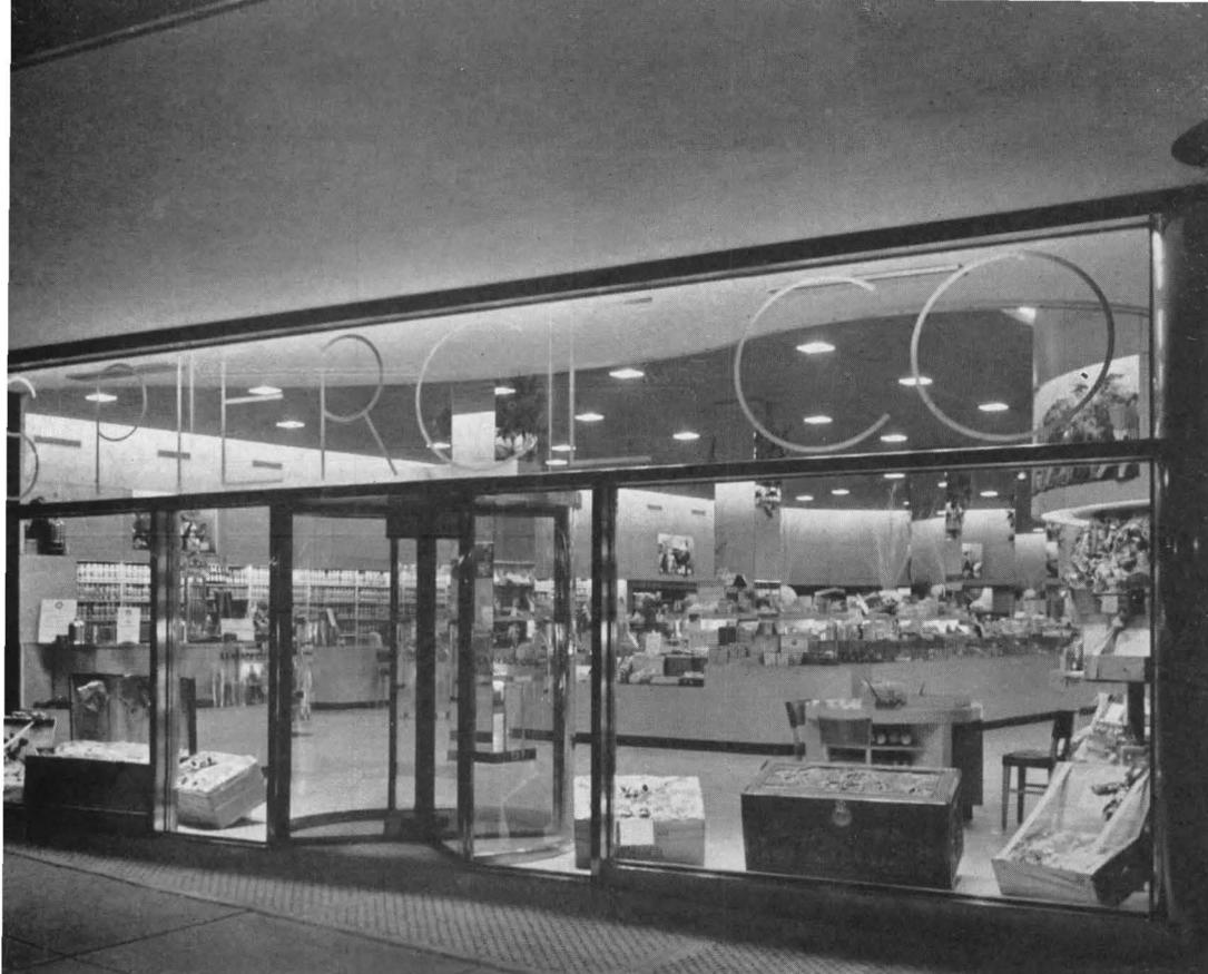
An off-center column in the facade suggested a display window in the smaller part and an all-glass store front and entrance displaying the activity of the whole store. To save space the office building entrance was incorporated with the store front. A cantilever marquee extends across the full front, its white soffit being softly floodlighted
