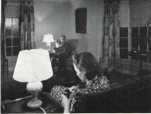
Figure 2: Brightness-contrasts of the work (sewing or reading) and the background cause eyestrain and fatigue. This lighting may be satisfactory for conversation, but not for critical seeing
