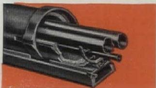
In this system, conduit is insulated from the exterior, but individual lines are not insulated from one another. A steam or hot water line can thus maintain temperature to keep liquids flowing in the other lines. Insulation is a diatomaceous earth lining, moulded and keyed to inside circumference of tile. May also be used with fibre insulation for steam heat, power and superheated steam. Applicable to Super-Tile and Cast Iron.
