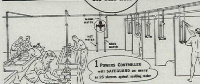
Use Powers thermostatic water mixing valves for Group Showers, Wash Sinks, Hot Water Line Control and Industrial Processes. Capacities up to 2,650 g.p.m. Write for Circular 3017. THE POWERS REGULATOR COMPANY, 2752 Greenview Avenue, CHICAGO—Offices in 47 Cities. 52
