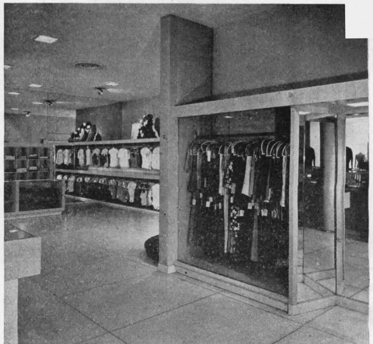
*Interior makes unusually quiet use of such elements as shadow boxes (view above); show cases have simple vertical slabs for legs. Column is covered with "woodweave." Floor is of cream-colored terrazzo. The intent was apparently to keep all elements uncluttered*
