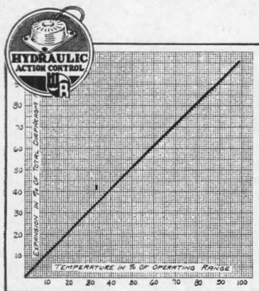
Notice, in the diagram at the left, how the expansion of the Hydraulic-Action diaphragm actually draws a straight line across the chart. This is because the force exerted by expansion or contraction under heat or cold is always *uniform*, and always predictable. That's another reason why White-Rodgers controls are easier to install and free of trouble.
