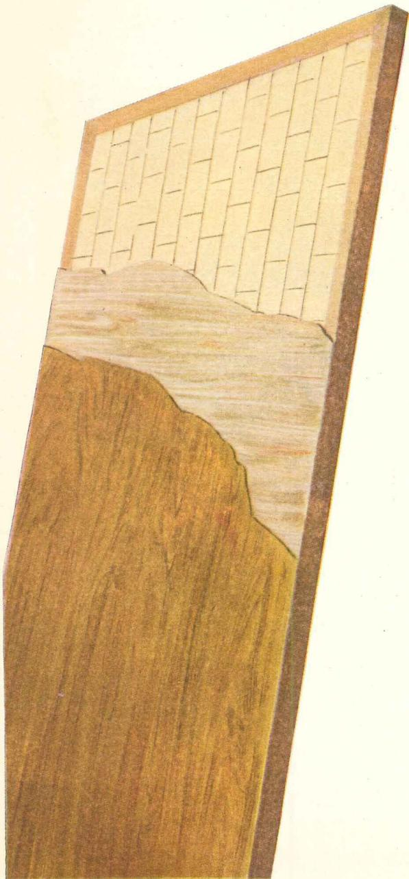
**H**ARD Michigan Maple faces over RODDISCRAFT cores and crossbanding welded into a solid, waterproof unit, under heat and pressure, by the RODDISCRAFT process, creates a door that will stand up under heavy traffic and harsh treatment.
