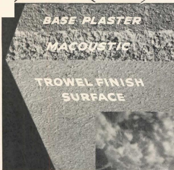
● Macoustic is applied over a base of gypsum plaster and saves the cost of the usual lime putty coat. May be troweled comparatively smooth or floated.
