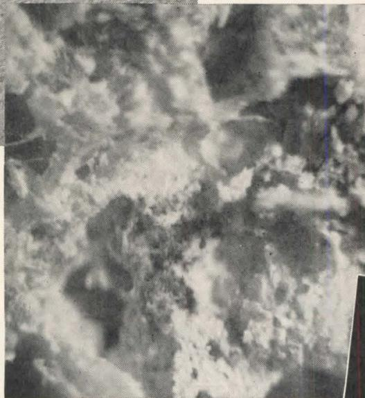
WHEN Gold Bond Macoustic is mixed with water, small gas bubbles form. After application, these bubbles burst, automatically creating millions of tiny sound-absorbing channels within the plaster which give this material its high acoustical efficiency.
