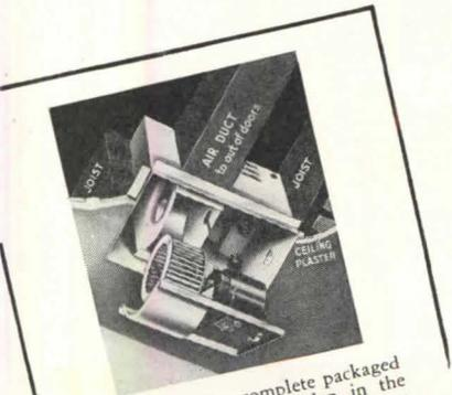
The Clipper is a complete packaged ventilator which is hidden in the ceiling. Only an inconspicuous "dripless" ceiling grille is visible, yet motor and blower assembly are instantly removed without tools for service.
