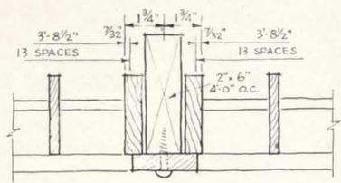
Full skylight detail was shown in ARCHITECTURAL RECORD for January, 1947. The wooden egg-crate light baffle to cut off sky-glare is here changed to go horizontally instead of following the roof. Note that its vanes are sloped to stop direct sunlight from a high southern sun.
