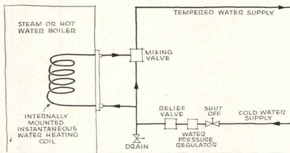
Above: Instantaneous hot water heater with internal coil
