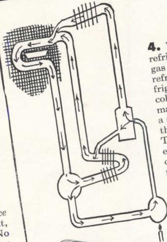
4. Why is Servel the different refrigerator? Because the small gas flame circulates a simple refrigerating liquid. This refrigerant supplies the constant cold that preserves food and makes plenty of ice cubes. Not a single moving part is used in the entire freezing operation. That means there's no machinery (no motor, no pump, no compressor, etc.) to ever need repair or replacement.
