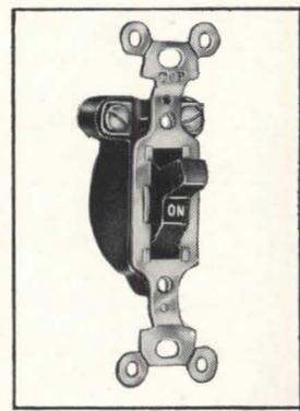
Now — an improved T-rated 10 ampere, 125 volt mercury switch, with all the advantages of silent, finger-tip action, increases your opportunity for better wiring jobs. Designed for top grade installation, this new Bryant specification-grade device widens mercury switch applications by meeting heavier load demands. Compact and totally enclosed in a Bakelite housing, it has large, readily accessible binding screws for easy top wiring. Available in single-pole, double-pole, 3-way and 4-way types.
