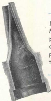
Independent laboratory tests prove that Flagg-Flow joints are stronger than the pipe itself. Illustrated is a torsion test. In a tensile test, the pipe failed at 65,000 pounds per square inch without harming the joint.
