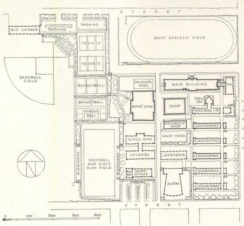
A fully-developed "finger-plan" school is easy for administrators to adapt to changing use. In the beginning it is natural to assign each wing or group of wings to a separate school group; but later, as groups shift in size, it is perfectly convenient to retain the basic zoning even though some wings are divided in two parts by the boundaries between zones
