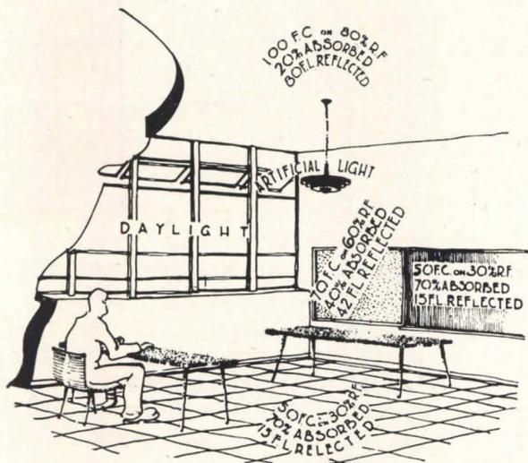
The reflection factor of ceilings, walls, chalkboards, floor and equipment determines to a large extent the degree of brightness balance that can be attained in a classroom. The efficient utilization of light energy, whether from daylight or artificial sources is dependent upon the reflection factor of the surfaces on which it falls
