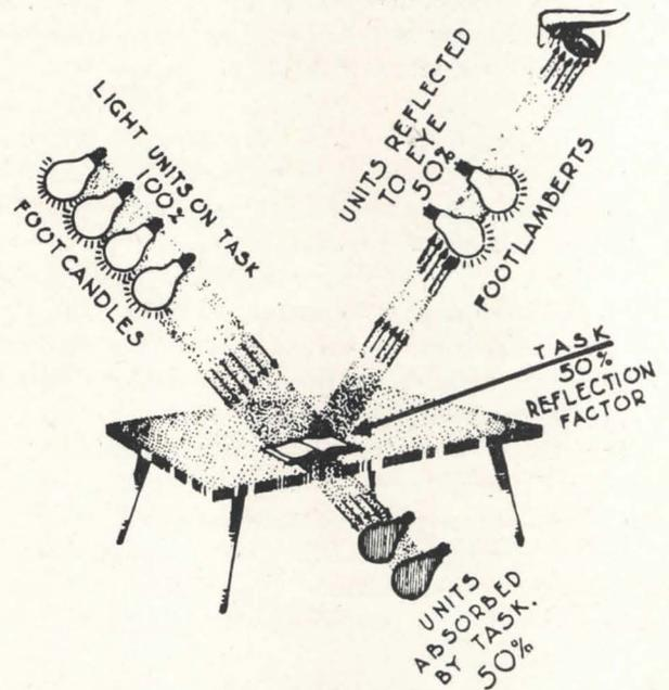
The light unit which activates the visual process is the footlambert. The task indicated above becomes visible because of reflected brightness. This reflected brightness is the product of the footcandle intensity and the reflection factor of the task. The footlambert, then, rather than the footcandle becomes the prize factor to consider in conditioning an environment for visual comfort and efficiency because it is the reflected brightness that we see and not the light falling upon the task
