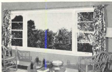
The new Curtis Silentite double-hung window unit is 20% more weather-tight than the famous original Silentite introduced in 1932. New construction includes floating weather-strips that press snugly against moving parts of window, yet permit easy operation. And, of course, Silentite has no weights or pulleys. Photo shows Silentite double-hung units flanking a Curtis picture window.
