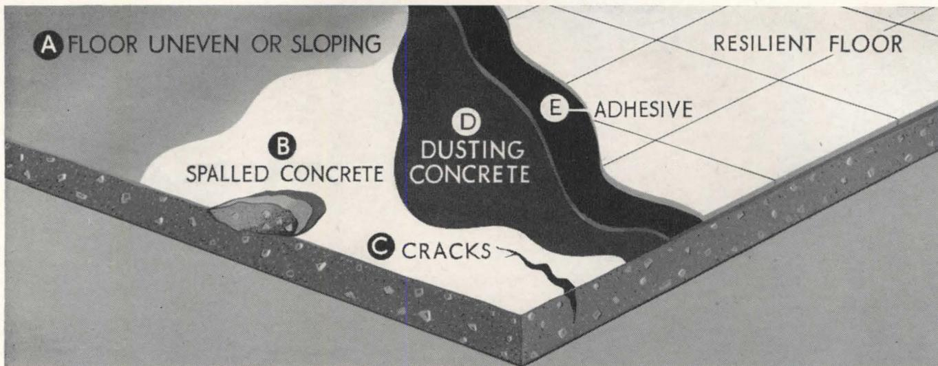
FIG. 1—This composite illustration shows the treatments necessary to correct the most common defects in old or worn concrete subfloors before the installation of resilient flooring. Uneven sections of the floor (A) are leveled with floor fill applied in the manner of a concrete topping. Holes
