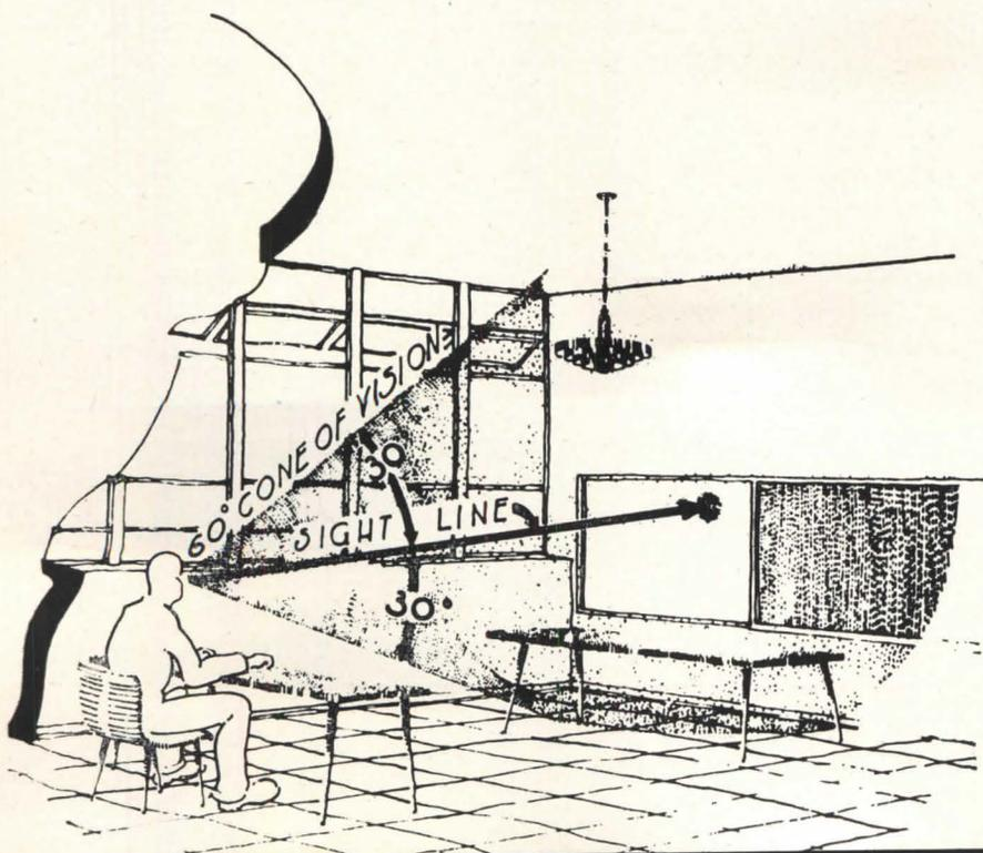
It is apparent from the illustration at left that the 60° cones include the major portion of the classroom even when the students are facing directly forward. This means that the entire classroom including the windows, lighting fixtures, ceiling, walls, floors, furniture and equipment should be conditioned to meet the requirements of brightness-difference recommended for the surrounding field
