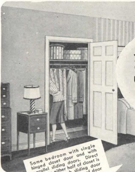
Same bedroom with single hinged closet door and with parallel sliding doors. Direct access to either half of closet is possible as each sliding door opens to opposite side of door frame. Note added floor space available with sliding doors.
