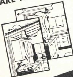
Specify Clipper for customer satisfaction. Mounts between ceiling joists above the stove. Vented out-of-doors through side wall or roof. The powerful squirrel cage blower (not a fan) keeps kitchen free of cooking grease and odors.
