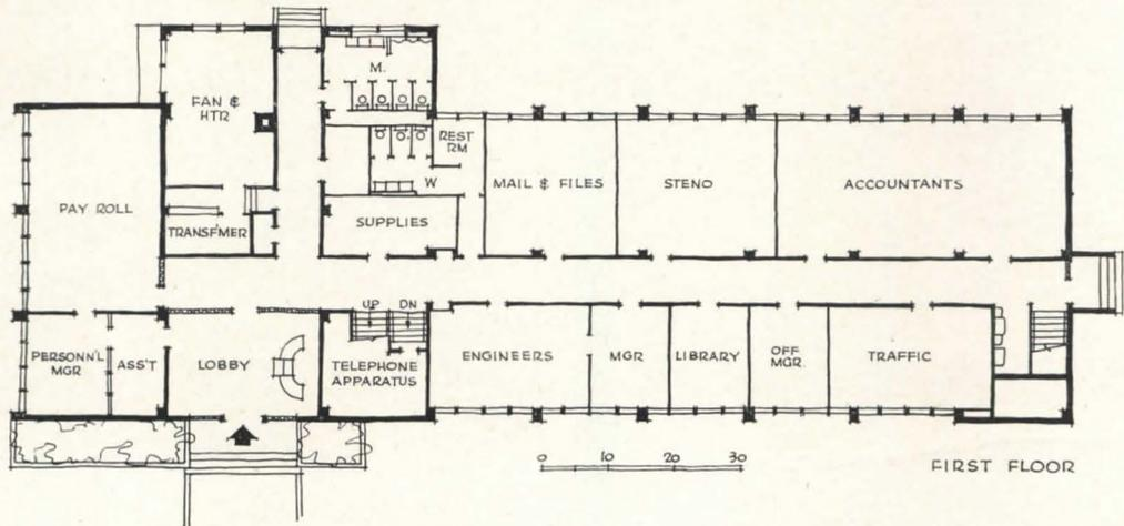
Both buildings (this one and the Martinez office building) were designed on a 4-ft. module — columns on 16-ft. centers, windows and fluorescent fixtures at 4 ft., air supply outlets 8 ft. on center from plenum chamber over corridors. Steel universal forms 2 by 3 ft. dictated the height of this concrete building at 12 ft. floor to floor. Overhangs are a continuation of the floor slabs
