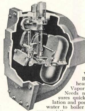
Webster Boiler Return Trap, heart of Webster Vapor Heating . . . Needs no motor. Assures quick steam circulation and positive return of water to boiler despite pressure variations.
