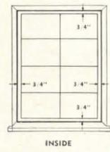
After the casement is erected, when installing inside trim, allow  $\frac{3}{8}$ " clearance around the casement on the interior so screens and storm windows may be installed.
