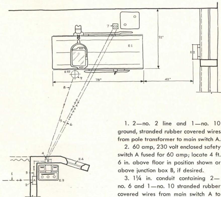
1. 2—no. 2 line and 1—no. 10 ground, stranded rubber covered wires from pole transformer to main switch A.
