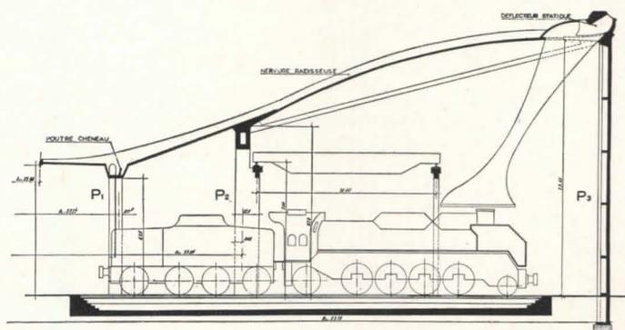
This fascinating roundhouse at Avignon, France, is remarkable for its ingenious and interesting structure, its functional architecture. The sections above show the special smoke-extraction system designed to remove smoke both from the building in general and from the engines in particular. The view at the top, left, shows the extraordinary lightness of reinforced concrete construction for which French engineers are so famous
