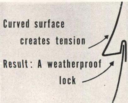
And this exclusive curved surface does even more. It is a deliberately engineered feature which makes this the strongest aluminum siding ever known. When lower edges are nailed down, the curve creates a tension which results in absolutely weathertight joints. And it creates beautiful clean lines.
