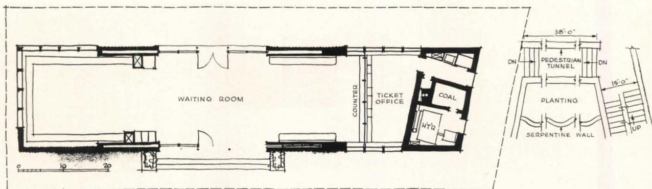
The plans are simple, and set a new standard for clean station design. An ample use of glass, which affords an almost uninterrupted vision of the platforms and train approaches from all parts of the buildings, has replaced the former unsightly bay windows common to older stations. All planning is very open, so that great crowds can pass through the station buildings rapidly without obstacles
