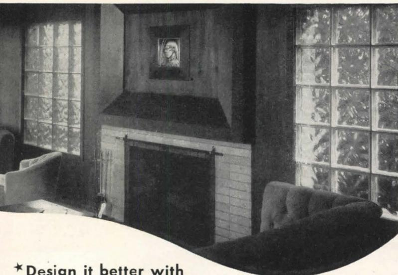
**AN AMPLE AMOUNT** of well-diffused daylight is admitted into this living room through the two panes of attractive Pittsburgh Corning Glass Blocks. The blocks can be used effectively to dampen outside noises—cut off unattractive views. And their insulating properties cut heating costs. 10 patterns to select from. Designer: Joseph J. Tarantino, Cleveland, Ohio.
