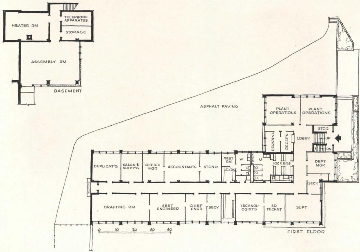
Office space can be subdivided at any 4-ft. window mullion, as the plan indicates; thus there could be an 8-ft. office ("secy" on plan), a 12-ft. unit for an executive, and so on upward to large open offices. As in the preceding building, columns are outside; there is nothing inside to interfere with placing of standard movable partitions in any desired position
