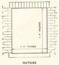
Rough openings should be plumbed and squared during construction and must be  $\frac{1}{4}$ " wider and  $\frac{1}{4}$ " higher than the overall dimensions of the casement frames. This permits installation without distortion.
