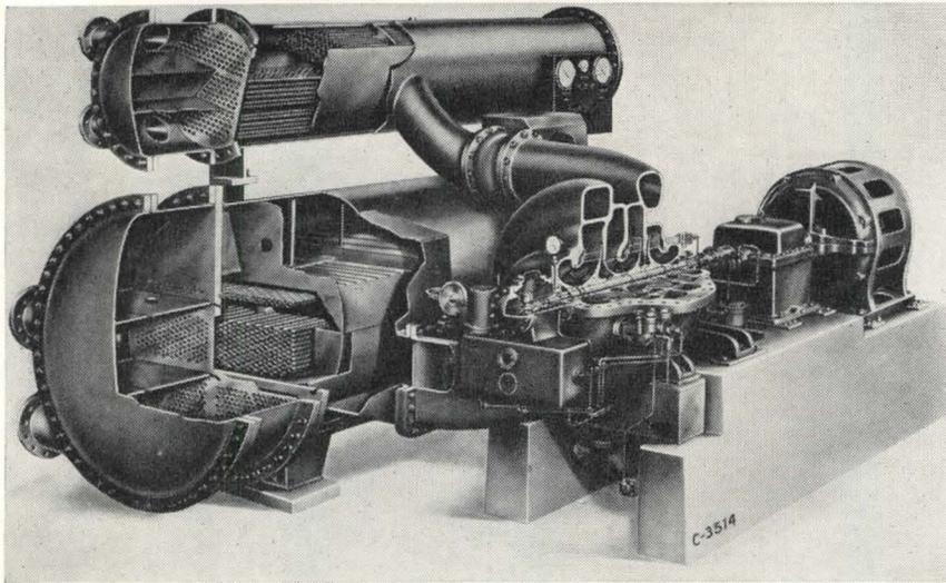
The use of "volute" in the design of the centrifugal compressor which forms a part of the Worthington Centrifugal Refrigeration System provides greater efficiency because the smooth, obstruction-free gas passages reduce friction and turbulence loss.
