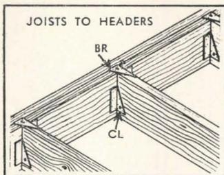
**1** Cheaper Than Ledgers—Trip-L-Grip eliminate cost of ledger strip, its placement and fastening. Cost of notching joists is eliminated. Joists are securely tied to beam or header.
