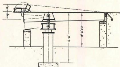
The loading operation is said to present a serious problem because (1) truck bed heights vary as much as 12 in.; (2) the truck bed moves up or down as loading or unloading progresses. The seriousness of the problem is said to have been increased with the use of power vehicles handling heavy loads.
