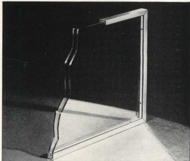
**HERE'S THE SECRET** of Twindow's insulating effectiveness. Two or more panes of Pittsburgh Glass separated by hermetically sealed air spaces. Entire unit is enclosed in a protecting frame of stainless steel.
