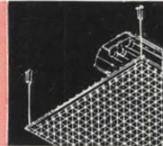
"Sky-Glo" is a system of channels, fittings and louvers of standardized sizes which makes it easy to fit a "Sky-Glo" ceiling to any size room. The simple, quickly assembled units reduce cost; actually "Sky-Glo" costs less than the usual conventional false ceiling.
