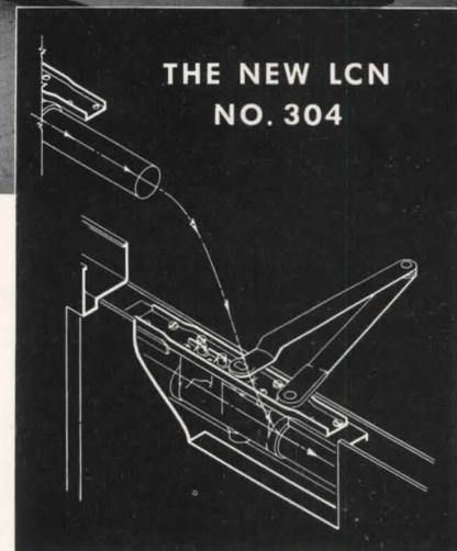
**NOW YOU CAN EQUIP THOSE INTERIOR METAL DOORS WITH EFFICIENT, LOW-COST LCN CLOSERS CONCEALED-IN-DOOR**
