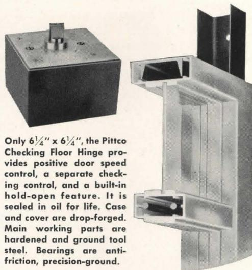
Only  $6\frac{1}{4}''$  x  $6\frac{1}{4}''$ , the Pittco Checking Floor Hinge provides positive door speed control, a separate checking control, and a built-in hold-open feature. It is sealed in oil for life. Case and cover are drop-forged. Main working parts are hardened and ground tool steel. Bearings are anti-friction, precision-ground.
