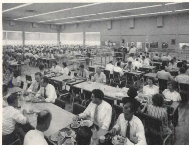
lighting, supplementing semi-continuous, recessed troffer fluorescent lighting, on 12- or 13-ft. centers in the suspended metal acoustic ceiling, 18 ft. above the floor. This installation maintains a general lighting level of 45 foot-candles. The ground floor is likewise illuminated by semi-continuous fluorescent units, to a general level of 25 foot-candles.
