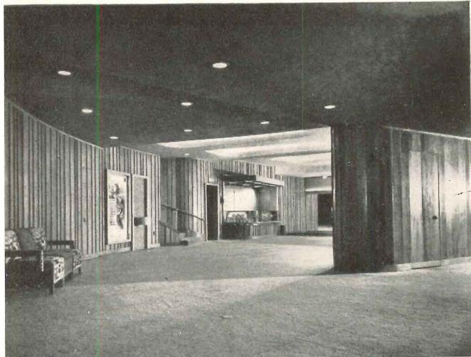
The lobby and stairwell walls, as well as the wainscot of the auditorium, are vertical cypress boards, random width, lapped joints, finished natural. The lobby is lighted indirectly near the entrance, and its ceiling steps down as one approaches the auditorium, the final portion having down lights which give adequate illumination without spilling light into the auditorium
