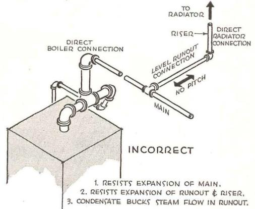
**CORRECT AND INCORRECT BOILER AND RADIATOR CONNECTIONS**
