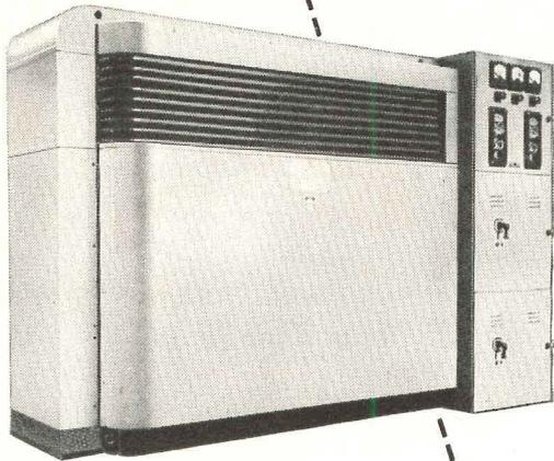
Load-center distribution keeps uneconomical low-voltage cable short, power loss low, voltage regulation high—In fact, here's a power-distribution idea that may bring you almost unbelievable savings in first cost, and at the same time make your system more flexible and expandable. Power is distributed at relatively high voltage to unit substations located near the load centers. There it is stepped down to utilization voltage and distributed to the loads via short feeders.
