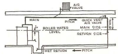
When return cannot be visible it may be buried in or below slab; coat outside of return with asphaltic paint; do not put return in water-bearing soil or cinders. Pit is required if system is to be drained.
