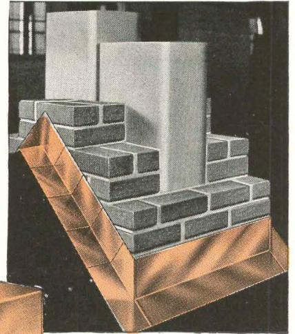
2 Cap flashing is made in two halves and may be shop-fabricated.
