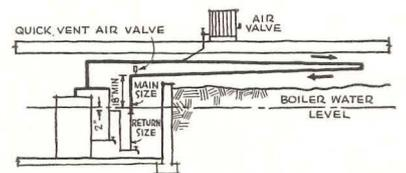
Space limitation may necessitate dry return; do not connect radiator runouts to it unless it is as high as main. Note position of quick-vent valve and minimum height of return above boiler water level.
