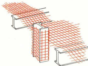
**First** it is the most efficient reinforcement. Its many small members of cold drawn, high yield-point steel fortify all parts of the concrete structure. Rolls and flat sheets of American Welded Wire Fabric provide continuous reinforcement in buildings, bridges, tunnels, etc. It can be wrapped around pillars, beams and girders, laid in steps, stairs and other irregular structural shapes.
