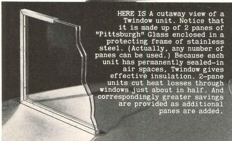
HERE IS A cutaway view of a Twindow unit. Notice that it is made up of 2 panes of "Pittsburgh" Glass enclosed in a protecting frame of stainless steel. (Actually, any number of panes can be used.) Because each unit has permanently sealed-in air spaces, Twindow gives effective insulation. 2-pane units cut heat losses through windows just about in half. And correspondingly greater savings are provided as additional panes are added.
