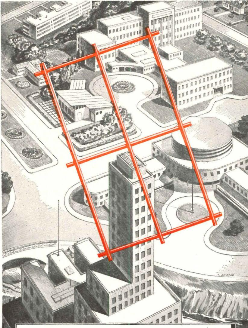
This sketch shows where American Welded Wire Fabric is used in modern concrete buildings. It reinforces walls, floors and roofs, can be draped over beams and girders and wrapped around pillars. Many uses of concrete in irregular structural shapes are made practical by American Welded Wire Fabric reinforcement.
