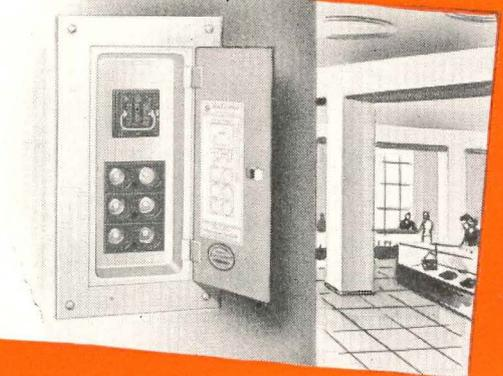
Ⓢ SEPF fuse-protected service equipment with safety-type Ⓢ Pulfuzswitch for main disconnect is ideal for residential or small commercial buildings. Available in standard enclosures for flush or surface mounting, and raintite for outdoors. With 30 or 60 ampere main connection, plug fuse branches, and extended feeder connection.
