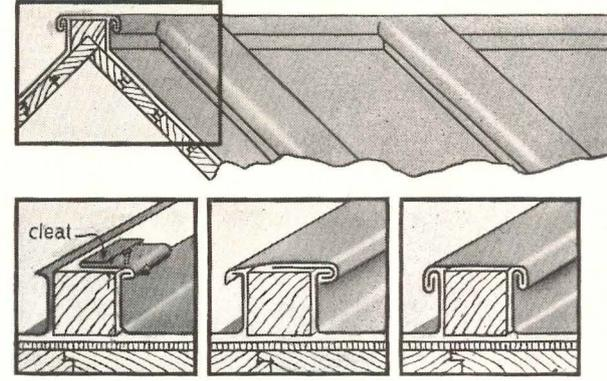
Standing Seam Construction Detail
