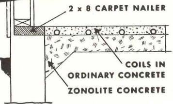
With Zonolite Concrete Aggregate your radiant heat jobs will assure rapid heating, better temperature control, and important fuel savings. Heat loss into the ground can be greatly reduced if you follow these simple steps:
