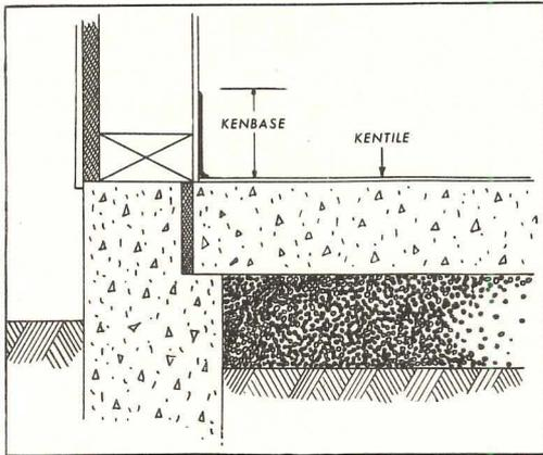
**Installs on concrete in direct contact with the earth**—All fillers, binders and pigments in Kentile have high resistance to the alkali found in concrete. And Kentile's asbestos filler assures insulation against the cold and moisture in concrete floors. Equally ideal for installation on radiant-heated concrete slabs.
