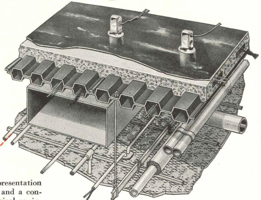
The cross-section is a condensed presentation of Q-Floor with suspended ceiling and a condensed visualization of the mechanical equipment required for a modern building. The drawing shows only equipment commonly installed between subfloor and ceiling. A modern building, also, must be a machine capable of accommodating any amount of electrical equipment above the floor.
