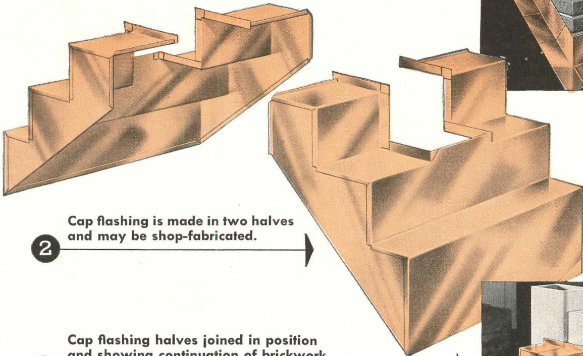
3 Cap flashing halves joined in position and showing continuation of brickwork.
