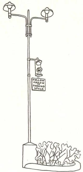
troller will immediately switch that light to red. Some control system of this type is particularly necessary when the aisles are as long as they are here, making it extremely difficult for the arriving motorist to see from one end if there are any empty stalls.
