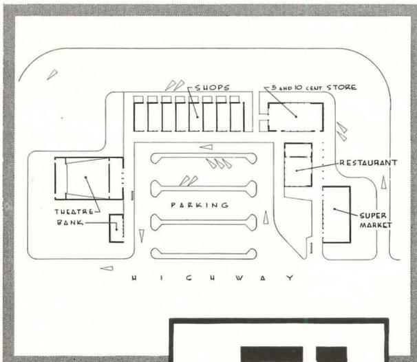
The shopping center above is designed around these six Luria units—five with 40-foot spans and 12-foot eave height, and one 80 feet wide with 20-foot eave height.
