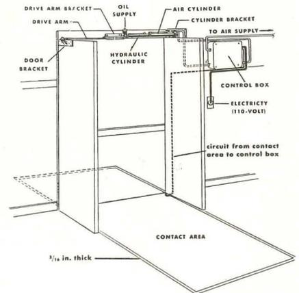
Door control uses no motors or gears
