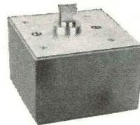
◀ COMPACT, EFFICIENT, laboratory-tested Pitteo Checking Floor Hinge. Especially developed for Pittsburgh Doorways. Has built-in door holder, positive door-speed control, separate checking control. Is sealed in oil for life.
