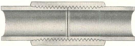
**SHERARDUCT COUPLING**—All surfaces and threads are Sherardized. Accurately undercut threads permit completely closed joints—no raw threads exposed—no gaps to interfere with the easy fishing of wires.
