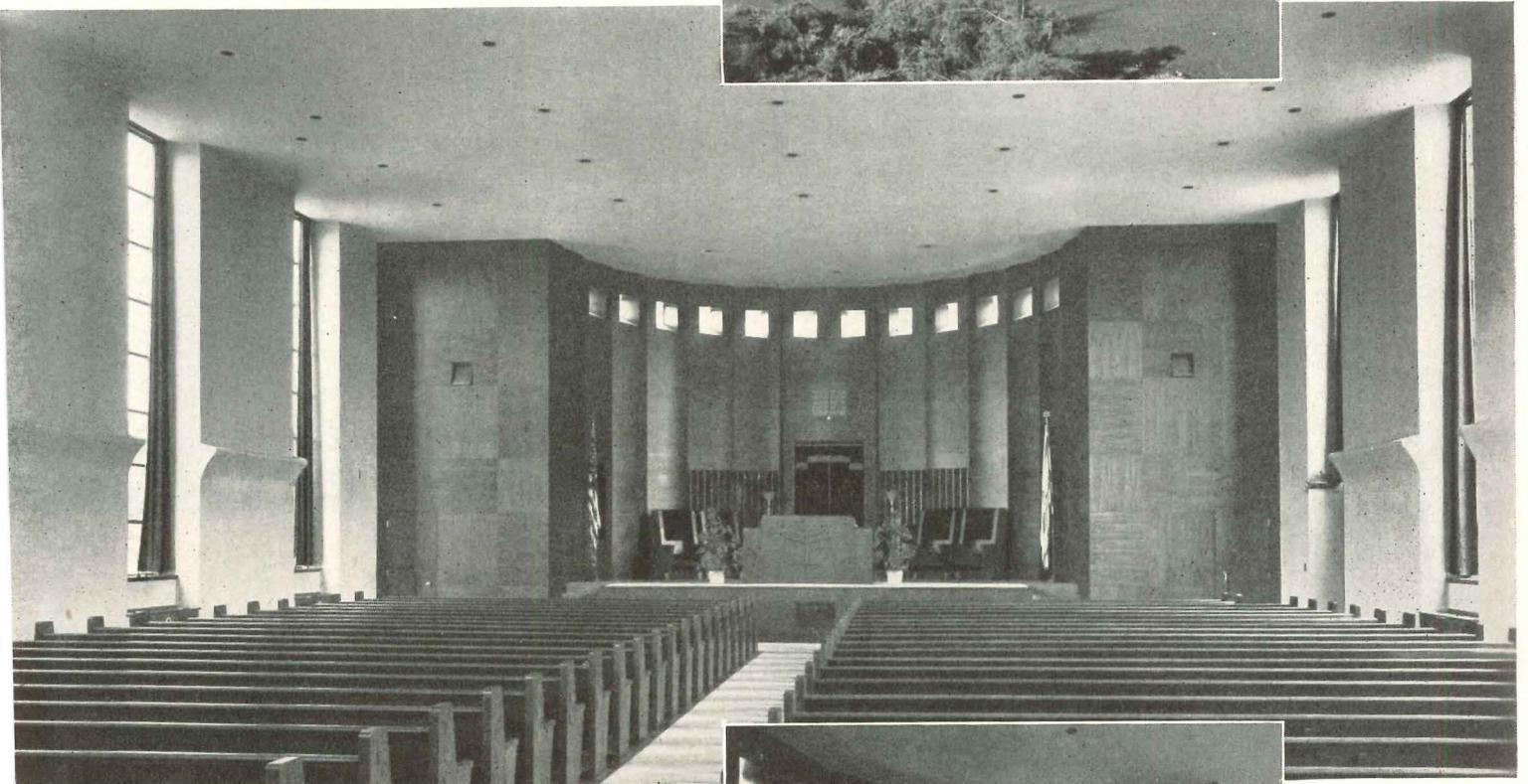
*The chapel has no projecting lighting fixtures; ceiling is light-studded and washed with indirect light from troughs between the windows along side walls. Paneled walls of the bima are walnut, stained and waxed. The 12 windows above Arc represent the 12 tribes of Israel*
