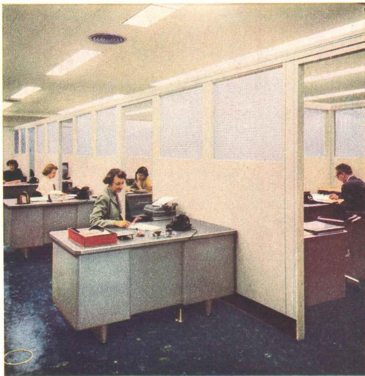
**Mills Walls** create pleasant, efficient environments. Baked-on enamel finishes require no maintenance but occasional washing to keep fresh new look. Air conditioning, light and phone lines are in separate lay-in raceways in panel connections, cornice, base.
