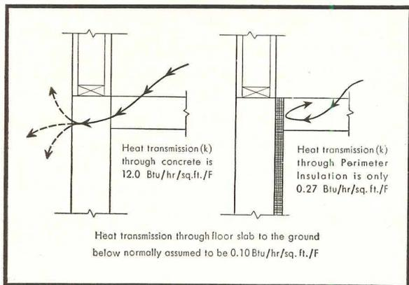
Fiberglas Perimeter Insulation prevents heat flow to cold outside air.
