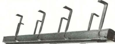
Truscon Slotted Inserts are attached to the forms and are completely imbedded in the concrete. Bolt can be moved along slot to any location, allowing wide variation in position. Used in ceilings, slabs, beams or columns.
