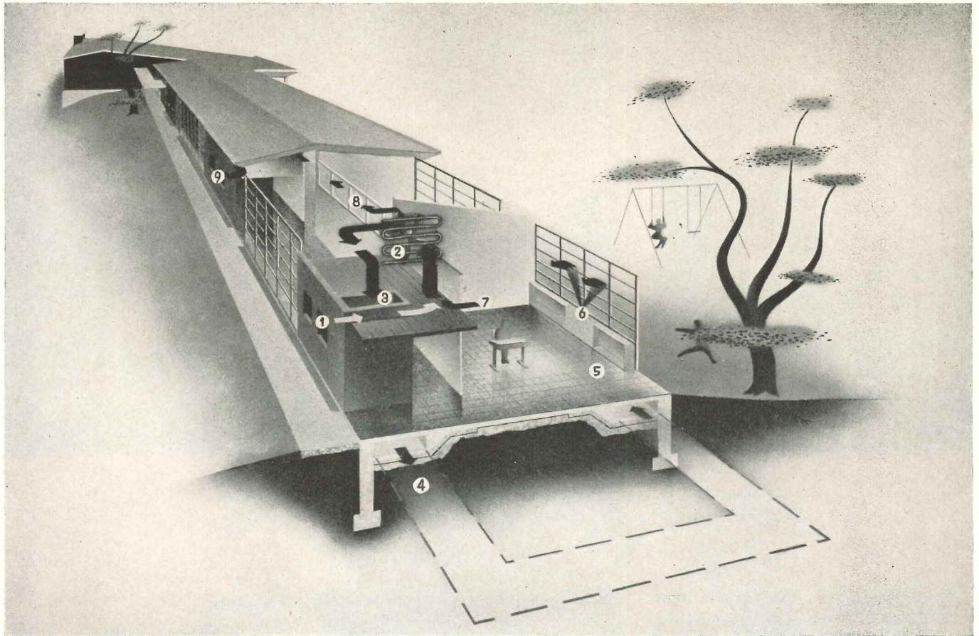
How the heating system operates: 1. Fresh air is taken in above exterior end door. 2. Air is drawn past steam heat coils by the fan. 3. Air leaves coils at 135F. 4. Air passes through concrete duct. 5. Air in duct keeps floor warm. 6. Air is thrown in front of cool glass area. 7. Half of air is recirculated (drawn from near ceiling). 8. Half of air is exhausted from classroom (drawn from near floor). 9. Air is exhausted to the outside
