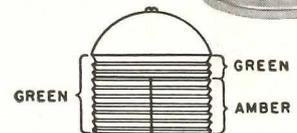
Construction of Pathfinder-head type prism lens combinations: 360°, 180°, or 3 prism 360° rings.
