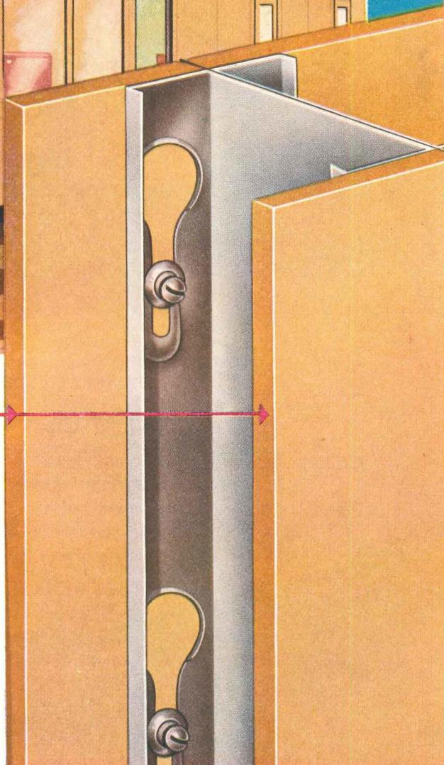
Cutaway of J-M Movable Wall construction. The  $\frac{7}{16}$ "-thick asbestos panels, on patented steel studding, are available in a light tan or light green. Note color is not a surface coating; it actually goes *all the way through* each panel.
