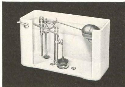
Interior view of Briggs Syphon Jet Closet Tank reveals latest design Anti-Syphon quiet operating flushing mechanism. This positive shut-off ballcock incorporates the latest type volume regulator, triple seal rubber ball, 1 1/8-inch overflow tank valve, large refill tube and positive quiet action at high or low pressures. Every part quality engineered for lasting dependability.
