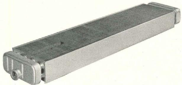
All steam passages are copper for long life and resistance to corrosion. The Nesbitt radiator is at the *top* of the cabinet away from the outdoor air intake for added freeze protection.
