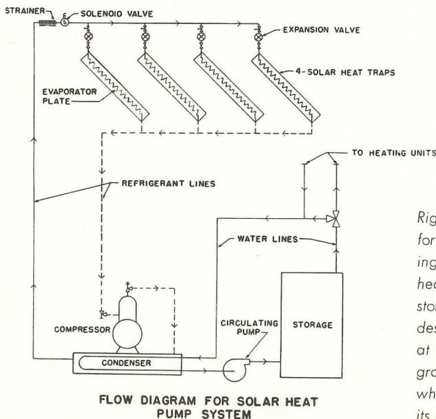
Right: some possible designs for sun-heated houses, showing variations in location for heat collectors and heat storage units, which were described by Prof. Anderson at the Symposium. Left: diagram of heat pump system which uses sun for part of its energy
