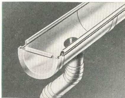
Reynolds 5" Half-Round Gutter, supplied with 3" Downspouts either plain round or corrugated. Allow one round downspout for each 700 sq. ft. roof area, one corrugated for each 600 sq. ft. Matched fittings as for Ogee. Available in either smooth or stipple-embossed finish.
