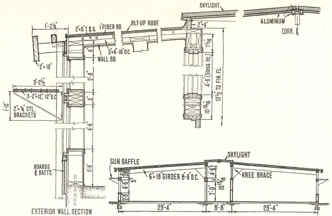
Section, details and photo show construction mostly of native wood, and method of borrowing light from interior corridor for classrooms either side. Each classroom wing will be a self-sufficient unit during normal school hours; only at recess, etc., will children have to use the outdoor, roofed corridors between wings
