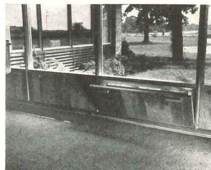
The complete unit may be obtained with frames of treated wood or extruded aluminum, and can be installed in frame or masonry walls or in construction combining both. Glazing may be single, double or triple plate glass. Heat loss is reduced by weather stripping and insulation. Both interior and exterior trim are furnished with the units, which are available in stock sizes or in made to order specifications. Solar Air-Flo, Inc., Dept. A., Elkhart, Ind.
