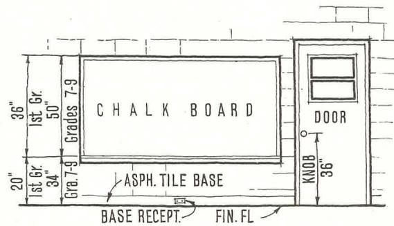
Typical classroom details. Above: section through washroom, with heights indicated for wainscotting, mirror and lavatory. Above right: heights of chalk board and door knob on typical wall elevation. Below right: arrangement of sink and wall cabinets
