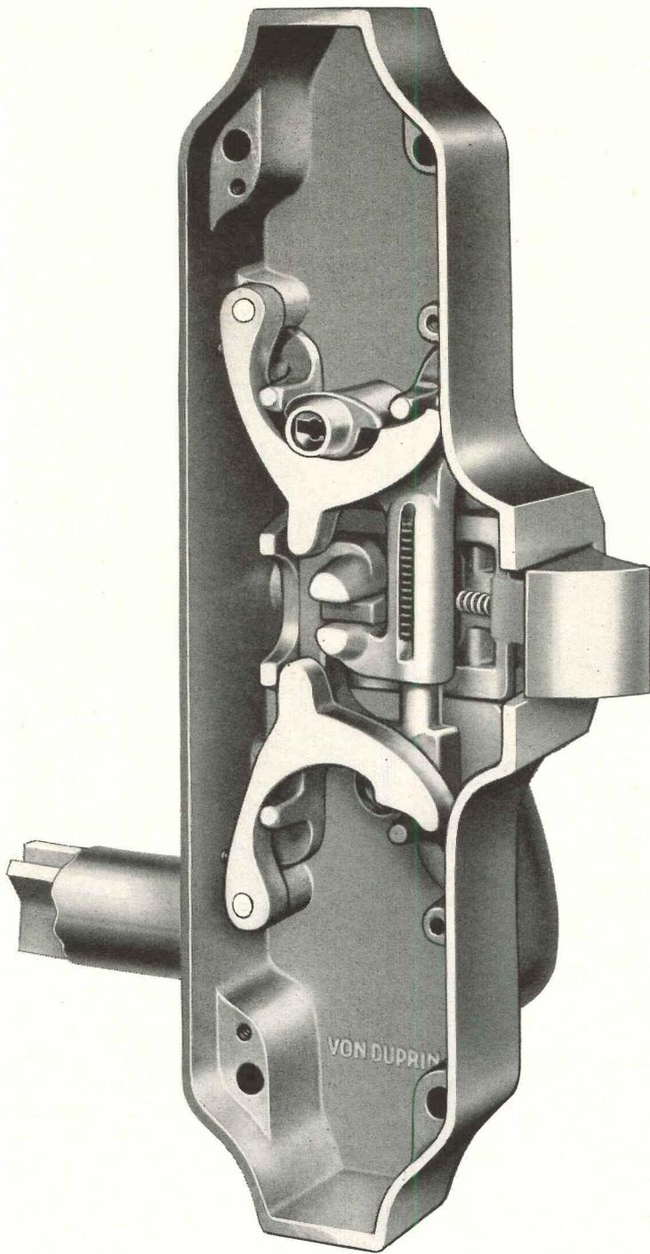
*Every part shown in this illustration of an A2 Von Duprin case is of drop-forged bronze except the two pins, the springs, the cross bar and its X-Bar reinforcement. The cross bar is of bronze tubing and the X-Bar of extruded bronze. Until science learns more about metals, there is no way to make a finer, tougher, more durable exit device.*
