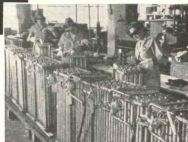
Attention to the many details that make up the completed unit typifies the Aerofin way. For instance, in this particular coil, careful brazing of the return tubes to the header plates assures leak-proof construction.
