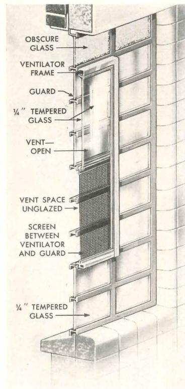
New window for mental hospitals has integral detention grill, provision against self-injury. Top left: typical installation. Right: component parts. Bottom left: detail showing method of holding glass in place
