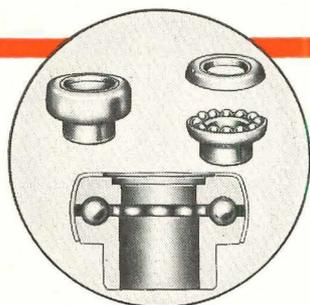
Exclusive Full-Jeweled Ball Bearing assembly consists of a movable and fixed raceway. When lateral thrust occurs, the movable raceway transmits the force directly to the bearings, which, in turn, are held firmly by the fixed raceway. Thus, the weight of the door is supported both laterally and vertically on ball bearings.
