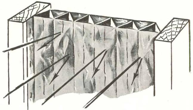
Tough aluminum is impervious to water vapor and yet has insufficient mass to extract heat from contacting air before reaching equilibrium in temperature with it. Colder air can support less vapor, and is an important cause of condensation.
