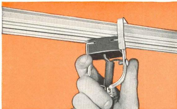
To tap off power at any point along the slot, simply insert twist-out plug and give it a 90° turn. Plugs are grounded on steel casing before contacts touch bus bars; narrow-access slot protects operator.
