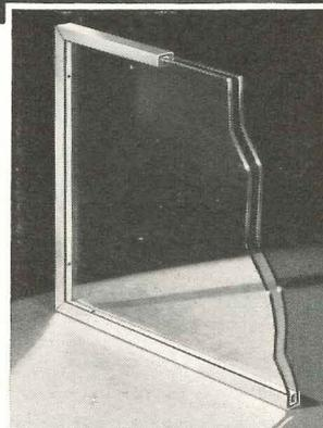
**HERE'S** the construction of a Twindow unit, using two panes of Pittsburgh Polished Plate Glass. The hermetically-sealed air space between the panes provides effective insulation which minimizes downdrafts, cuts heat loss through windows, reduces condensation. Insulation is even more efficient when three or more panes are used. Forty-seven standard Twindow sizes are available, adaptable either for wood or steel sash.
