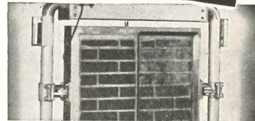
This photo shows continuous streams of water being directed from the top onto two brick panels, one of which has been treated with CRYSTAL.
