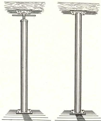
Plastic-covered columns are fabricated for either temporary or permanent supports
