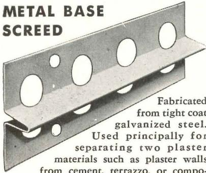
Fabricated from tight coat galvanized steel. Used principally for separating two plaster materials such as plaster walls from cement, terrazzo, or composition base, and separating a cement wainscot from ordinary plaster. Another function is to give a permanent straight edge to which both trades work.
