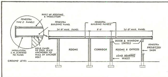
Interlocked Panels are simply welded to small plates mounted on top of concrete block walls.
