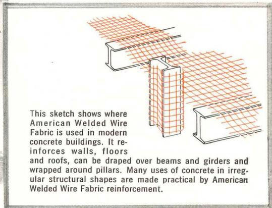
This sketch shows where American Welded Wire Fabric is used in modern concrete buildings. It reinforces walls, floors and roofs, can be draped over beams and girders and wrapped around pillars. Many uses of concrete in irregular structural shapes are made practical by American Welded Wire Fabric reinforcement.
