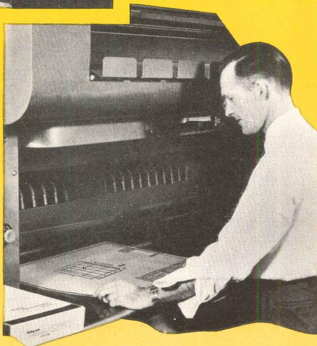
**How positive photographic intermediates are produced.** Kodagraph Autopositive Paper is exposed in Sikorsky's direct-process machine . . . processed in standard photographic solutions. No negative step . . . no darkroom handling—a revolutionary, economical operation that speeds print service to all departments!
