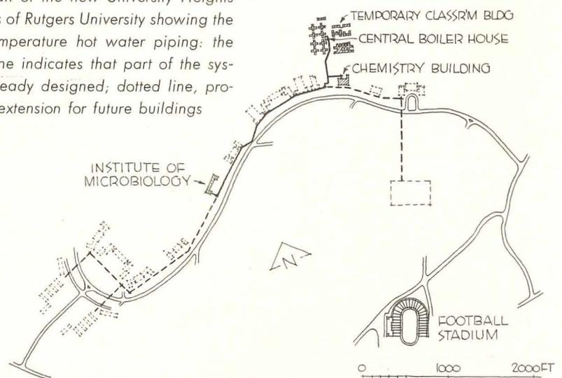
\*Design features proposed by the American Hydrotherm Corp. were incorporated in this distribution system, and the boilers were designed according to their specifications.
