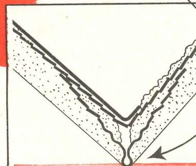
Here's why Super-Ex corners are so long-lasting: note greater depth of plaster adjacent to bead area . . . spring fit adapts easily to any specified depth plaster ground — whether it be 3/4", or 1/2" . . . and solid metal that protects corner at point of greatest strain.
