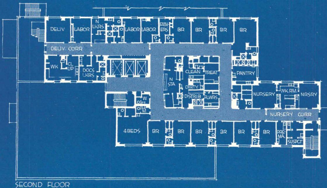
*A good illustration of the advantage of the T form in separating traffic and isolating departments*
