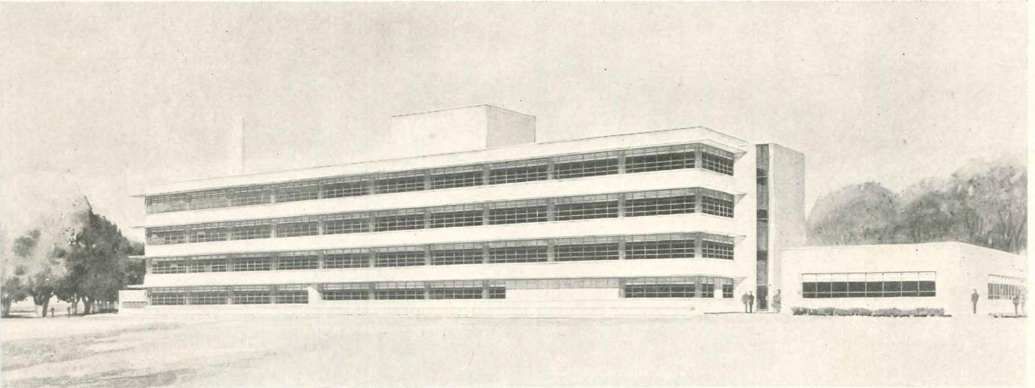
**A** MORE CONVENTIONAL SCHEME than others in this study, this hospital is an excellent example of the typical advantages of the T plan for a large hospital. Good separation of different traffic streams, good shielding of individual departments, positive control of visiting public, best orientation for patient rooms, isolation of noisier activities and deliveries — these are important merits of the T form.
