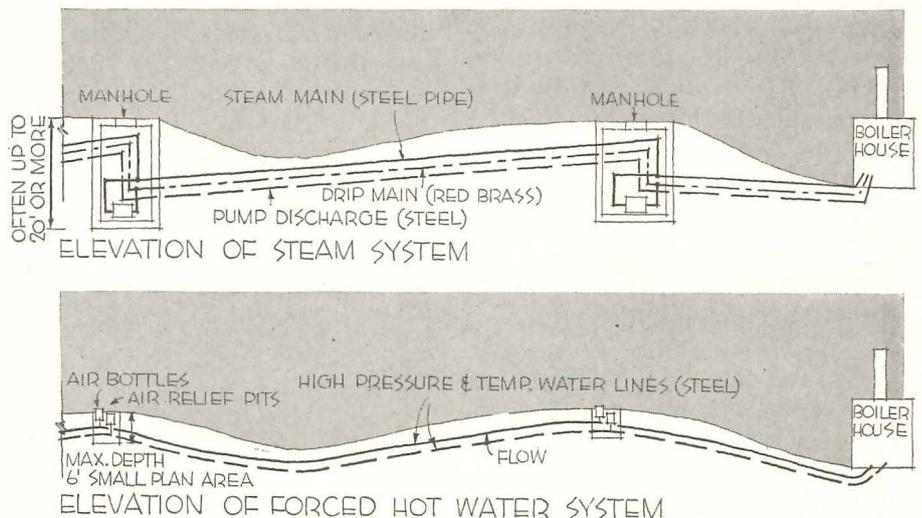
Hot water system piping can easily follow the contour of the land—the circulating pump takes care of any changes in elevation. With steam systems, pipe lines must be pitched down in the direction of flow to drain properly, and must be dripped at all low points. Red brass is usually used for drip mains to cut down on the amount of erosion. Red brass for the large steam main would be too expensive
