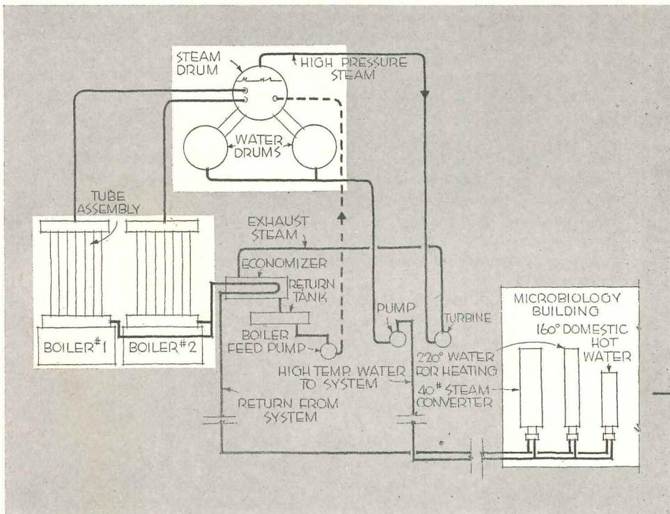
Schematic diagram of the high-temperature hot water system for Rutgers University. High-temperature water flows from drums to steam or medium-temperature hot water convertors in each building. High-pressure steam operates the turbine-driven circulating pumps. The return water is preheated by the exhaust steam
